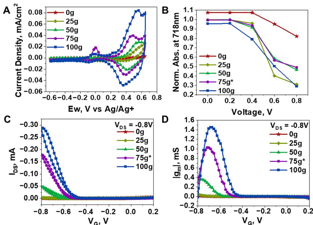
**Fig. 4** Electrochemical performance of polymers (A) cyclic voltammograms in 0.1 M LiPF<sub>6</sub>, and (B) corresponding spectro-electrochemical absorbance at 718 nm. (C) Characteristic transfer curves and (D) corresponding transconductance values from OECT devices based on *mg*-IID polymers with 0.1 M LiPF<sub>6</sub> as the electrolyte.
