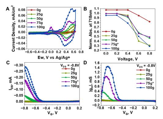
Fig. 4 Electrochemical performance of polymers (A) cyclic voltammograms in 0.1 M LiPF<sub>6</sub>, and (B) corresponding spectro-electrochemical absorbance at 718 nm. (C) Characteristic transfer curves and (D) corresponding transconductance values from OECT devices based on mg-IID polymers with 0.1 M LiPF<sub>6</sub> as the electrolyte.
