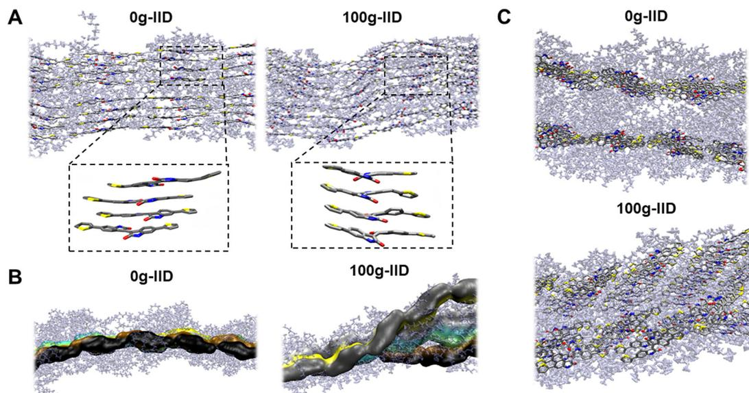
**Fig. 3** MD simulation snapshots of the **mg-IID** polymers with highlighted backbones. (A) Difference in the  $\pi$ -stacking of the two polymers, with zoomed packing of the IID cores. (B) Arrangement of the packed polymer chains in a plane. (Each color represents the backbone for the same chain) (C) Difference in the lamellae stacking of the two polymers.
