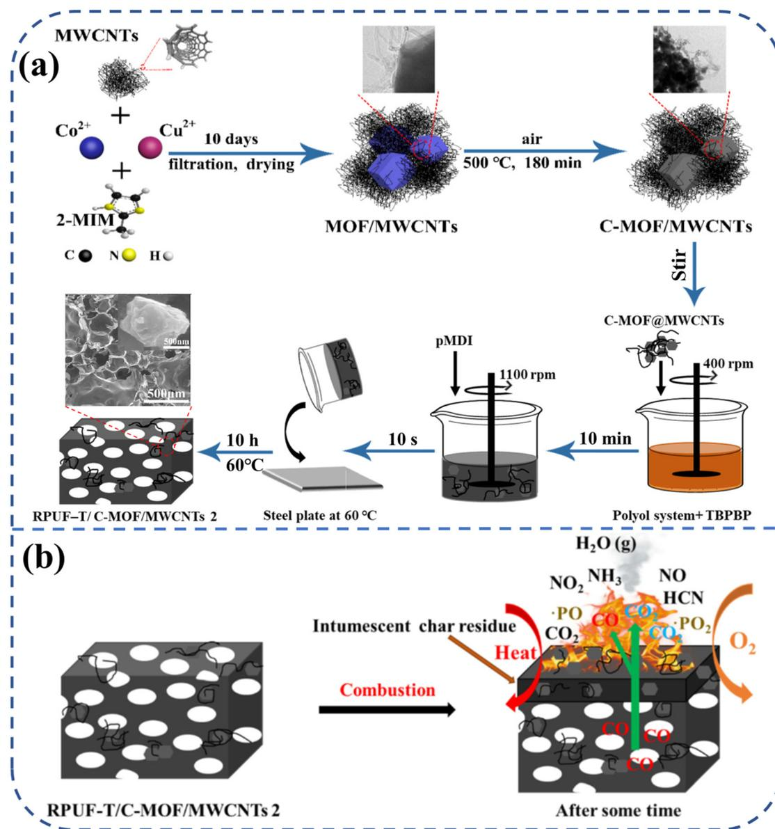
**Fig. 8** (a) Schematic diagram of preparation and (b) flame retardant mechanism of bio-based RPUF-T/C-MOF/MWCNTs. Free copyright reserved MDPI 2022.
