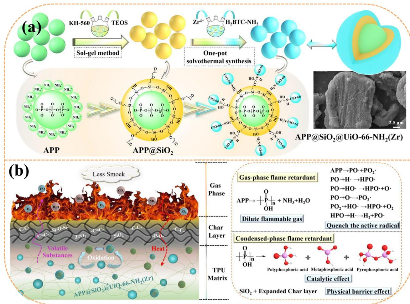
Fig. 5 (a) Schematic of the production route of APP@SiO<sub>2</sub>@UiO-66-NH<sub>2</sub>(Zr). (b) Flame retardant mechanism of the TPU composites. Reproduced with permission from ref. 64, copyright reserved Elsevier 2023.
