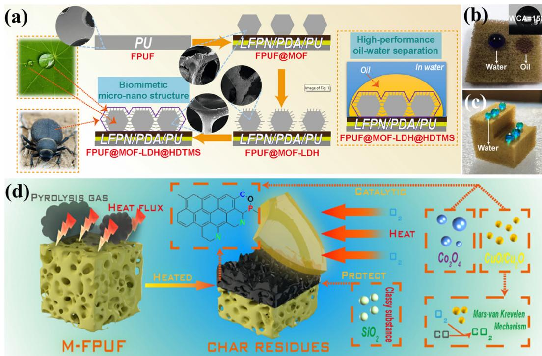
**Fig. 13** (a) Schematic of FPUF@MOF-LDH@HDTMS bionic structure and oil–water separation mechanism; (b and c) wettability of FPUF@MOF-LDH@HDTMS; (d) flame retardant mechanism of FPUF composite. Reproduced with permission from ref. 94, copyright reserved Elsevier 2023.
