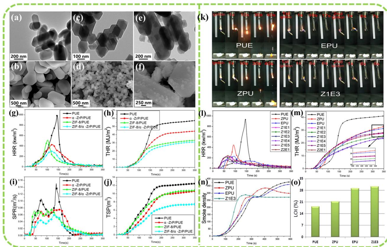
**Fig. 3** TEM and SEM images of (a and b)  $\alpha$ -ZrP, (c and d) ZIF-8, and (e and f) ZIF-8/ $\alpha$ -ZrP; (g) HRR, (h) THR, (i) SPR and (j) TSP curves. Reproduced with permission from ref. 46, copyright reserved Wiley 2018. (k) UL-94 vertical burning test; (l) HRR, (m) THR, (n) smoke density, and (o) LOI curves for pure PUE and PUE composites ( $Z_xE_y$  denotes the ZIF-8 to EG ratio of  $x:y$ ). Reproduced with permission from ref. 47, copyright reserved Wiley 2019.
