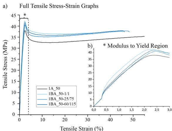
**Fig. 9** (a) Stress–strain graphs of annealed ISO 527 1A tensile bars tested at an elastic crosshead velocity of  $50 \text{ mm min}^{-1}$  compared to ISO 527 1BA tensile bars tested at velocities based on dimensional ratios of 1BA/1A (Table 2); (b) a zoom-in of the modulus to yield region. Tables with the specific averages can be consulted in the ESI S1–S4.†
