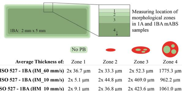
**Fig. 8** Thickness of different morphological zones in mABS 1BA tensile bars manufactured via injection molding with different injection speeds or mold types to obtain different degrees of orientation.
