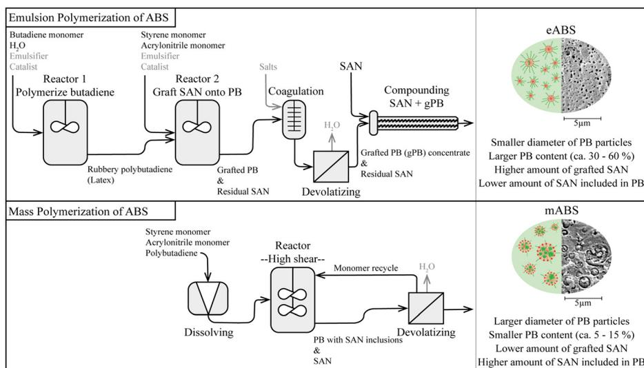
**Fig. 2** Morphological differences for eABS and mABS, based on SEM images made from Terluran HI-10 eABS and the investigated Magnum 3404 mABS of this research, linking these differences to the production process; in mABS for simplicity only one reactor shown.
