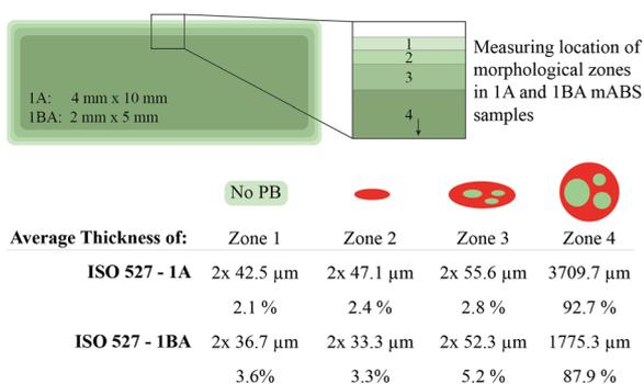
**Fig. 7** Measuring location to define the thickness of different zones within ISO 527 - 1A and ISO 527 - 1BA samples which were injection molded at  $60 \text{ mm s}^{-1}$ , with cross-sectional dimensions of respectively  $4 \text{ mm} \times 10 \text{ mm}$  and  $2 \text{ mm} \times 5 \text{ mm}$ .
