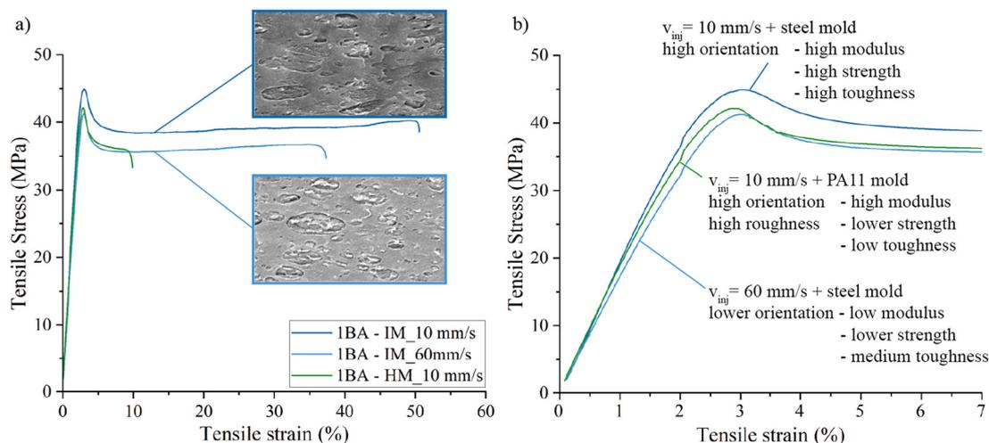
**Fig. 11** (a) Full tensile response of 1BA tensile bars injection molded in a steel mold at  $60 \text{ mm s}^{-1}$  (light blue line), in a steel mold at  $10 \text{ mm s}^{-1}$  (blue line) and in a MJF PA11 mold at  $10 \text{ mm s}^{-1}$  (green line) and (b) zoom-in of the elastic deformation area. Tables with the specific averages can be consulted in ESI (S7–S9).†
