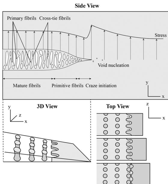
**Fig. 3** The general principle of craze formation and propagation in the absence of (rubber) particles (e.g. pure SAN; conventional crazing). The image of 3D and top view are based on the work of Kramer *et al.*,<sup>21</sup> while the side view is based on the work of Estevez *et al.* and Van Krevelen and Nijenhuis.<sup>23,24</sup> With rubber particles an analogous presentation is provided in Fig. 4.
