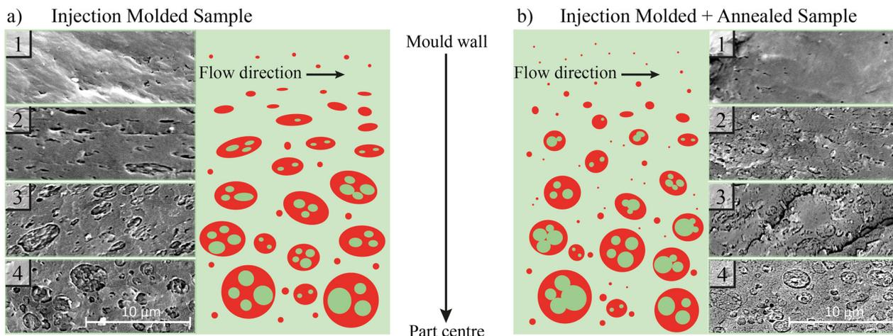
**Fig. 6** General morphology considering distribution and orientation for ISO 527 1BA test bars made of mABS via (a) injection molding at  $60 \text{ mm s}^{-1}$  and (b) with subsequent annealing at  $110 \text{ }^\circ\text{C}$  for 5 hours.
