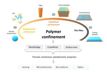
Fig. 1 Schematic framework of this perspective: from the fabrication of confined polymers to their properties and applications.
