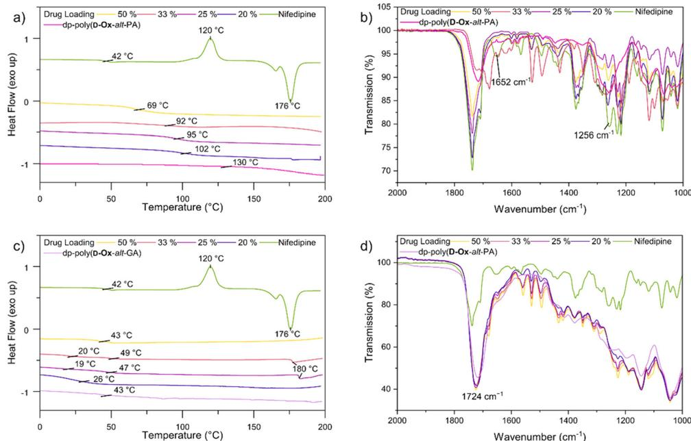
**Fig. 4** DSC spectra (exo up, second cooling cycle), 20 °C min<sup>-1</sup> of nifedipine ASDs with (a) dp-poly(*D-Ox-alt-PA*) (–) and (c) dp-poly(*D-Ox-alt-GA*) (–). FTIR spectra between 2000 and 1000 cm<sup>-1</sup> of nifedipine ASDs with (b) dp-poly(*D-Ox-alt-PA*) and (d) dp-poly(*D-Ox-alt-GA*) at 50% w/w (–), 33% w/w (–), 25% w/w (–), 20% w/w (–).
