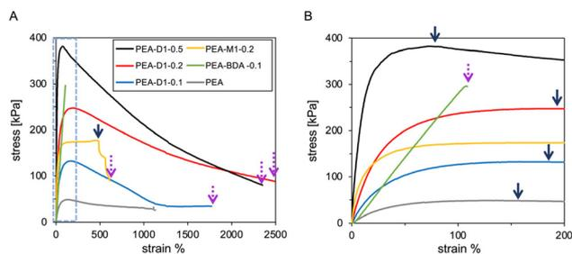
**Fig. 2** Stress-strain curves of PEA-D1, PEA-M1, PEA-BDA, and PEA by tensile tests at a rate of 1.0 mm s<sup>-1</sup> (A) and enlarged view at comparatively low strains (dashed line) (B). The concentration of the cross-linker was 0.1 (for D1 and BDA), 0.2 (for D1 and M1), and 0.5 (for D1) mol%. Arrows indicate elastic fields (solid lines) and fracture points (dashed lines).
