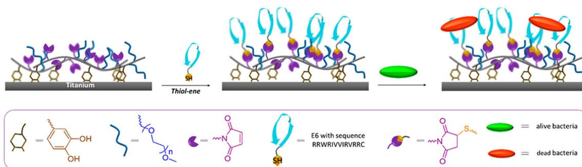
**Fig. 9** Schematic illustration of an AMP-conjugated thiol-reactive polymeric coating on a TiO<sub>2</sub> surface to fabricate an antimicrobial coating. Adapted with permission from Gevrek *et al.*<sup>51</sup> Copyright © 2019 American Chemical Society.
