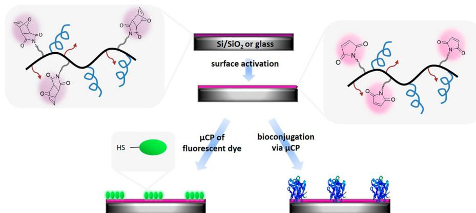
**Fig. 16** Fabrication of a thiol-reactive polymer-based thin film coating for sensing and biomolecule immobilization. Adapted with permission from Gevrek *et al.*<sup>127</sup> Copyright © 2017 American Chemical Society.
