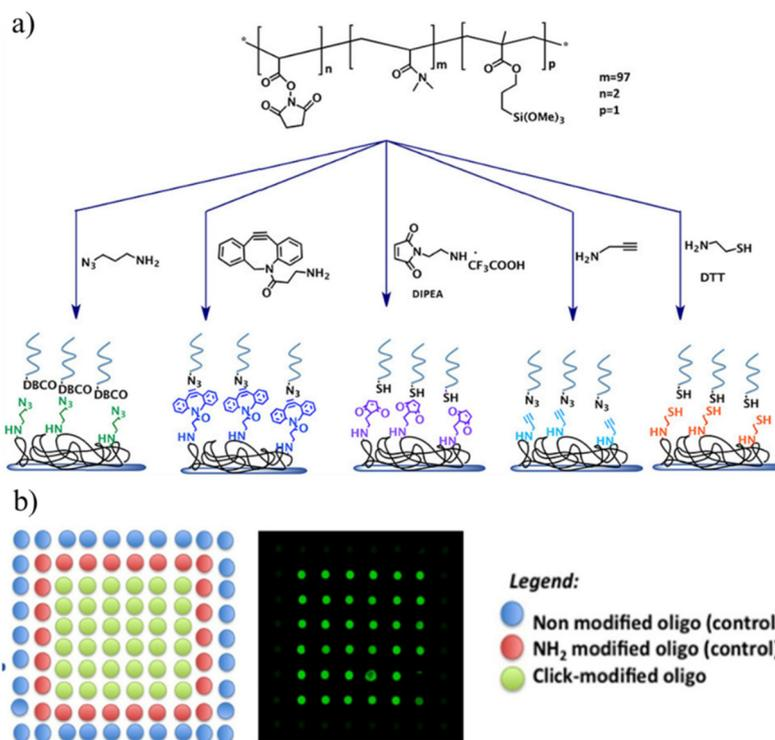
**Fig. 15** (a) Fabrication of clickable polymer coatings via post-polymerization modification for microarray technology and (b) schematic representation of the oligonucleotides immobilized on the surfaces, coated with the 'click' copolymers. Adapted with permission from Sola *et al.*<sup>109</sup> Copyright © 2016 American Chemical Society.
