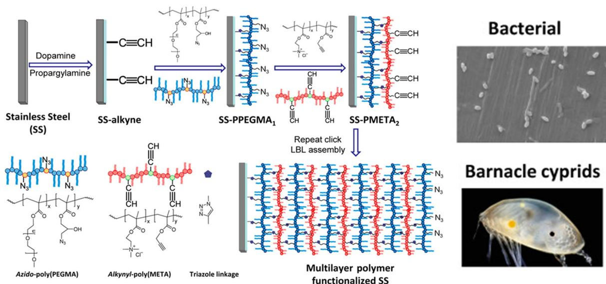
Fig. 4 Schematic illustration of antifouling and antibacterial polymer multilayer coating fabrication *via* layer-by-layer 'click' deposition. Adopted with permission from Yang *et al.*<sup>26</sup> Copyright © 2012 American Chemical Society.
