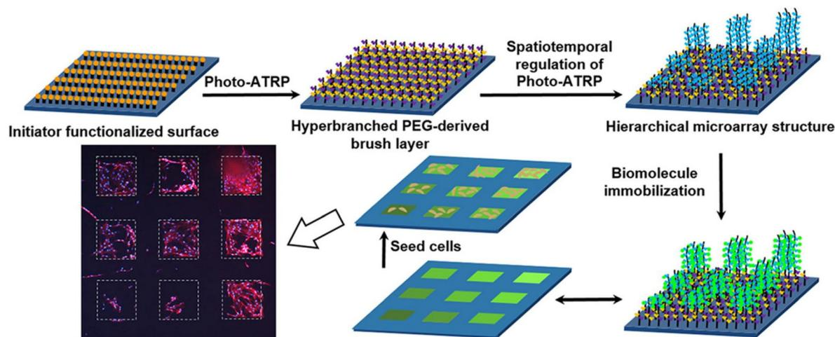
**Fig. 19** Fabrication of PEG-derived brush micropatterns for cellular microarray platforms. Adapted with permission from Zhao *et al.*<sup>140</sup> Copyright © 2020 Elsevier.
