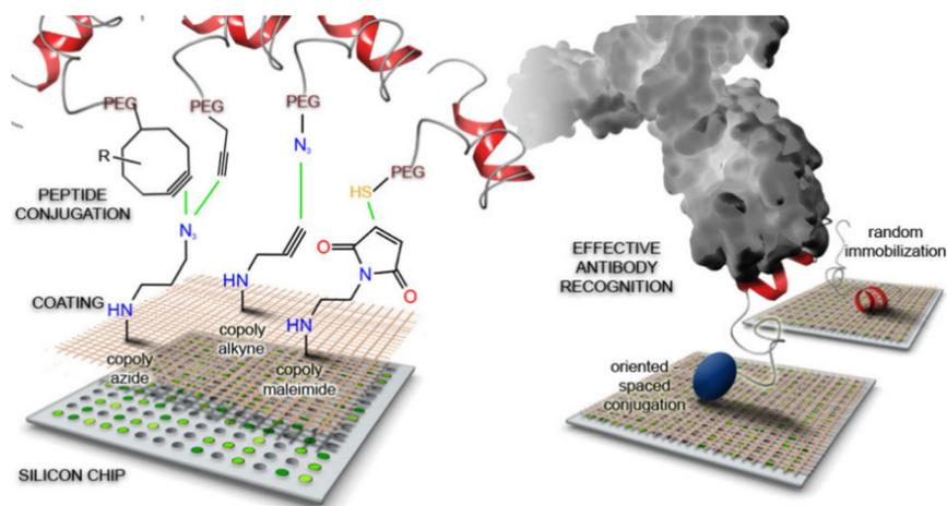
Fig. 14 Schematic illustration of peptide conjugation onto a 'clickable' polymer-coated silicon chip for effective antibody recognition. Adapted with permission from Gori *et al.*<sup>108</sup> Copyright © 2016 American Chemical Society.
