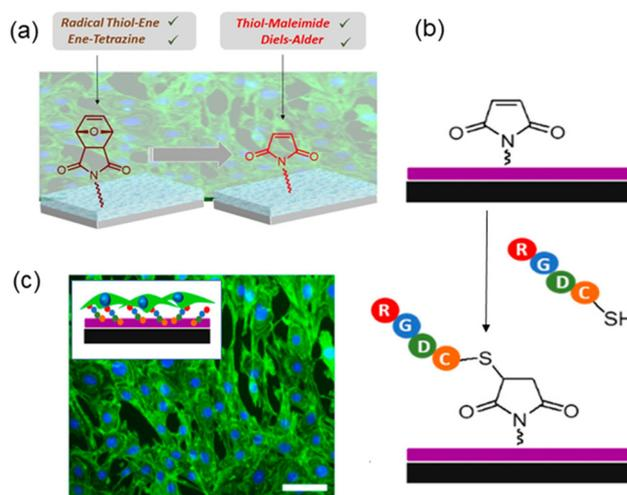
**Fig. 11** (a) Fabrication of a maleimide containing hydrogel coating on a titanium surface; (b) schematic representation of the RGDC conjugated hydrogel coating for cellular attachment and proliferation; (c) NIH-3T3 cell proliferation on the RGD-conjugated hydrogel coating. Reprinted with permission from Gevrek et al.<sup>80</sup> Copyright © 2020 by the authors. Licensee MDPI, Basel, Switzerland.
