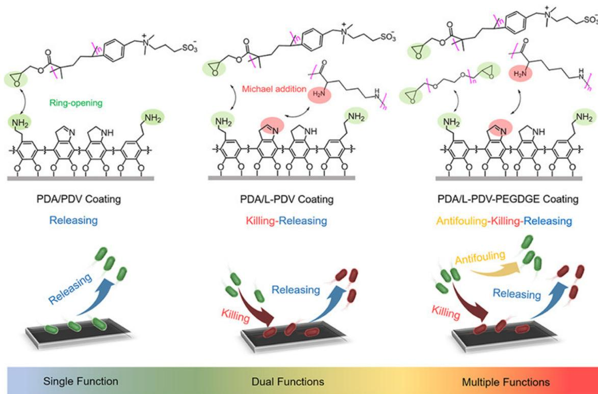
**Fig. 7** Schematic representation of mussel-inspired polymeric coatings realizing functions from single to multiple antimicrobial mechanisms. Three functional polymers, *i.e.*, polylysine, diethylene glycol diglycidyl ether (PEGDGE), and poly[glycidylmethacrylate-*co*-3-(dimethyl(4-vinylbenzyl) ammonium)propyl sulfonate] (poly(GMA-*co*-DVBAPS)), were selected. Adapted with permission from Mao *et al.*<sup>36</sup> Copyright © 2021 American Chemical Society.
