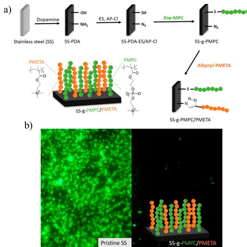
**Fig. 6** (a) Schematic illustration of fabricating binary polymer brush coatings on stainless steel surfaces via 'click' reaction; (b) fluorescence microscopy images of pristine SS and SS-g-PMPC/PMETA brushes after exposure to *S. aureus*. Adopted with permission from Xu *et al.*<sup>34</sup> Copyright © 2017 American Chemical Society.
