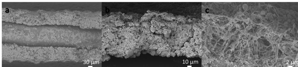
**Fig. 2** Cross-sectional SEM images showing (a) top and bottom of fractured PI coated NMC electrode. The middle layer is Al current collector, onto which the cathodic material was deposited. (b) PI coated NMC electrode with PI layer present on the top surface. (c) PI coating morphology displaying a network of particles with characteristic bead-on-string architectures.
