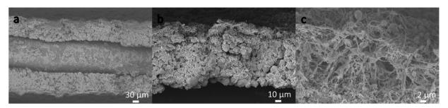
Fig. 2 Cross-sectional SEM images showing (a) top and bottom of fractured PI coated NMC electrode. The middle layer is Al current collector, onto which the cathodic material was deposited. (b) PI coated NMC electrode with PI layer present on the top surface. (c) PI coating morphology displaying a network of particles with characteristic bead-on-string architectures.
