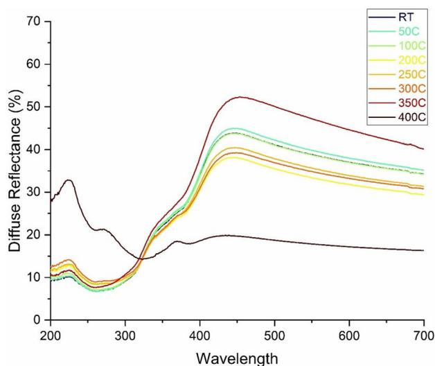
**Fig. 3** Diffuse reflectance UV-Vis spectra of SLED PI films on a Si substrate, illustrating the impact of temperature on film porosity. The PI was initially sprayed at RT, then thermally treated for ~10 minutes at each temperature increment, followed by RT UV-Vis spectral analysis for each temperature.
