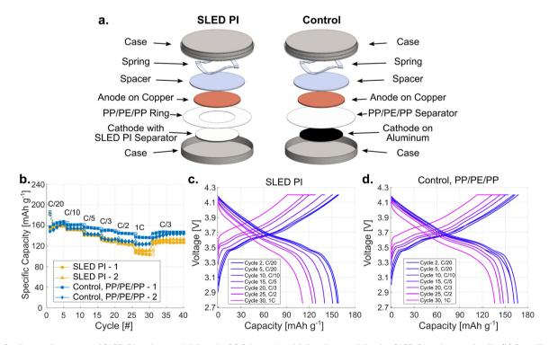
Fig. 5 Cycling performance of SLED PI and control full-cells. (a) Schematic of full-cell assemblies for SLED PI and control cells. (b) Specific capacity as a function of cycle number and C-rate. Hollow markers indicate charge capacity and filled markers indicate discharge capacity. Voltage profiles for the different C-rates for (c) a SLED PI full-cell and (d) a control sample with only a PP/PE/PP separator.
