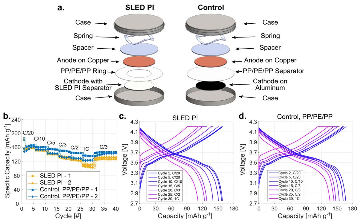
**Fig. 5** Cycling performance of SLED PI and control full-cells. (a) Schematic of full-cell assemblies for SLED PI and control cells. (b) Specific capacity as a function of cycle number and C-rate. Hollow markers indicate charge capacity and filled markers indicate discharge capacity. Voltage profiles for the different C-rates for (c) a SLED PI full-cell and (d) a control sample with only a PP/PE/PP separator.
