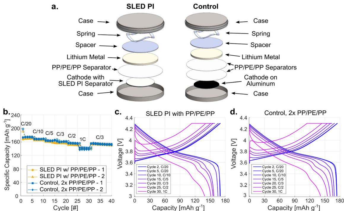
**Fig. 4** Cycling performance of SLED PI and control half-cells. (a) Schematic of half-cell assemblies for SLED PI and control cells. (b) Specific capacity as a function of cycle number and C-rate. Hollow markers indicate charge capacity and filled markers indicate discharge capacity. Voltage profiles for the different C-rates for (c) a SLED PI half-cell and (d) a control sample with only PP/PE/PP separators.
