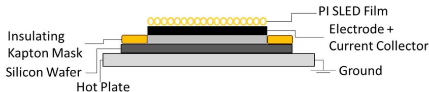
**Fig. 1** Illustration of the SLED film deposited onto an electrode. The use of a Kapton tape film mask improves coating uniformity and coverage by redirecting the electrostatic field lines of the spray onto the electrode.
