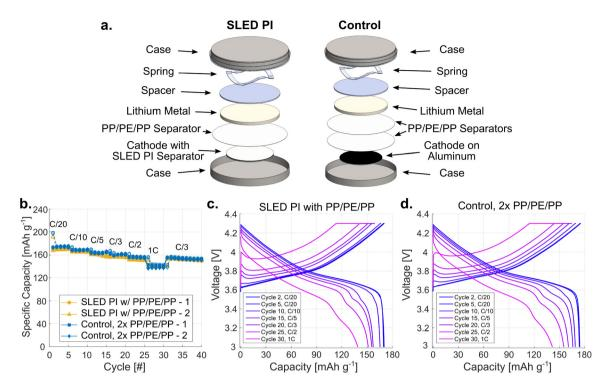
Fig. 4 Cycling performance of SLED PI and control half-cells. (a) Schematic of half-cell assemblies for SLED PI and control cells. (b) Specific capacity as a function of cycle number and C-rate. Hollow markers indicate charge capacity and filled markers indicate discharge capacity. Voltage profiles for the different C-rates for (c) a SLED PI half-cell and (d) a control sample with only PP/PE/PP separators.
