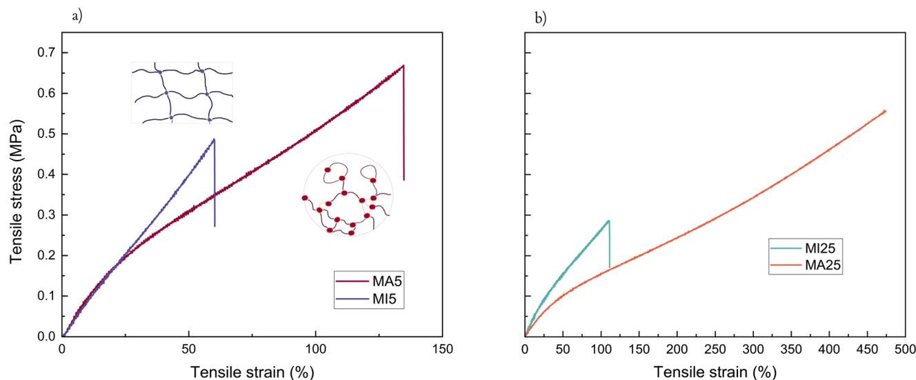
Fig. 4 Tensile test of the four network samples where (a) short-chain networks (MA5 v MI5, illustration inset of the two hypothesized network structures), and (b) long-chain networks (MA25 v MI25).
