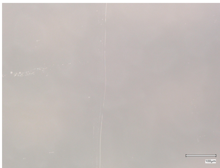
Fig. 8 Optical microscopy at 400x magnification of MA25 cross-linked network with an imposed cut visible but healed after self-healing for 24 h under room temperature.
