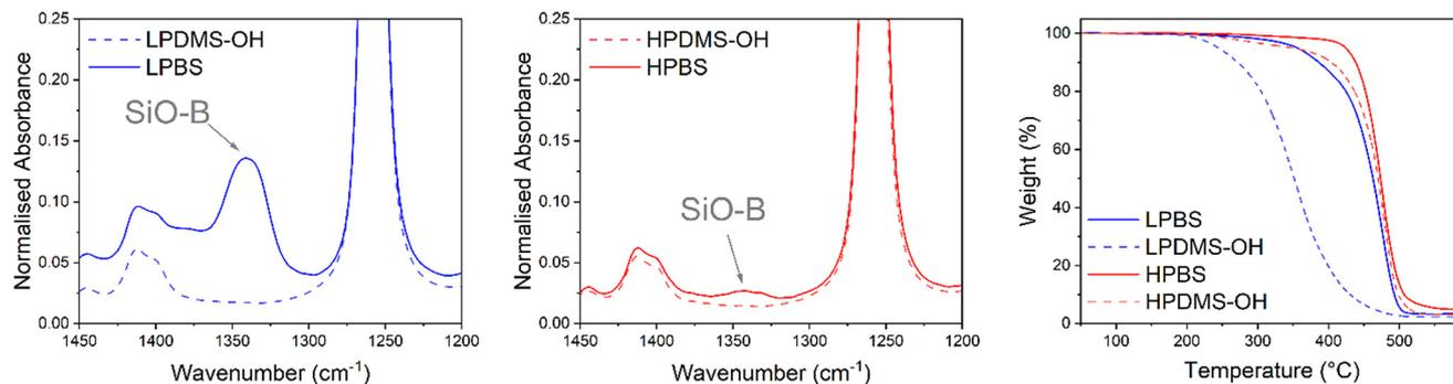
**Fig. 2** (Left & middle) Region of the FTIR spectrum showing the SiO–B stretch for LPBS (blue) and HPBS (red) compared to LPDMS-OH (dashed blue) and HPDMS-OH (dashed red). Each spectrum is normalised to the Si-CH<sub>3</sub> stretch at 1258 cm<sup>-1</sup>. (Right) TGA thermogram of LPBS (blue), LPDMS-OH (dashed blue), HPBS (red) and HPDMS-OH (dashed red) recorded at 10 °C min<sup>-1</sup> under a nitrogen atmosphere.
