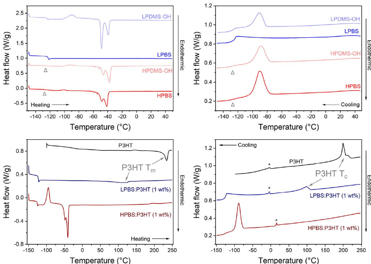
**Fig. 5** (Left column) Second heating and (right column) first cooling cycles of P3HT, PDMS-OH and PBS polymers, as well as PBS : P3HT blends recorded at a scan rate of  $10\text{ }^{\circ}\text{C min}^{-1}$  under a helium atmosphere. The light grey arrowhead indicates the  $T_g$  for HPDMS-OH and HPBS. The peaks marked with a star are measurement artefacts.
