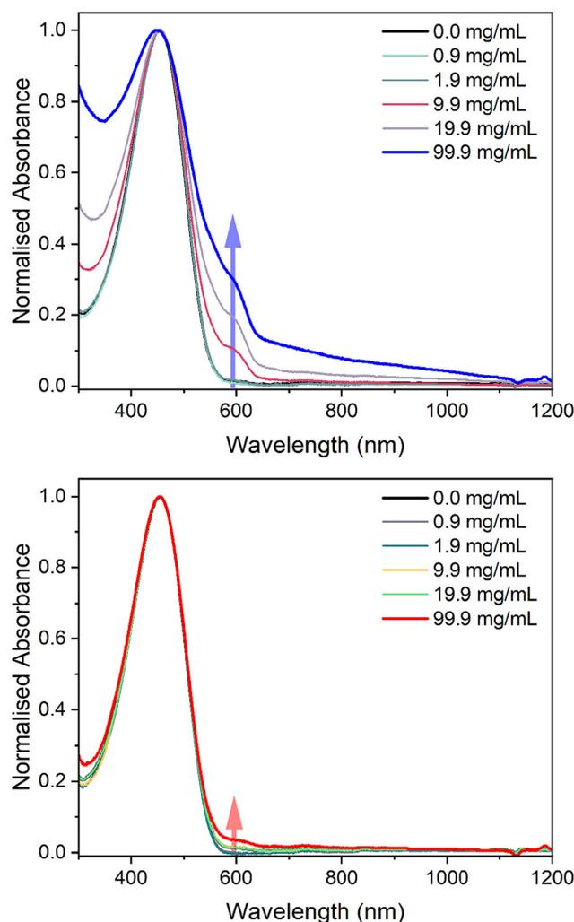
**Fig. 4** Normalised solution UV-vis absorbance spectra of LPBS : P3HT (top) and HPBS : P3HT (bottom) blends in chlorobenzene with an increase in the concentration of PBS with a constant concentration of  $0.1 \text{ mg mL}^{-1}$  P3HT. The spectra have been normalised to the  $S_0$  to  $S_1$  transition at 458 nm. The arrows highlight to the reader the P3HT aggregation peak at around 600 nm.
