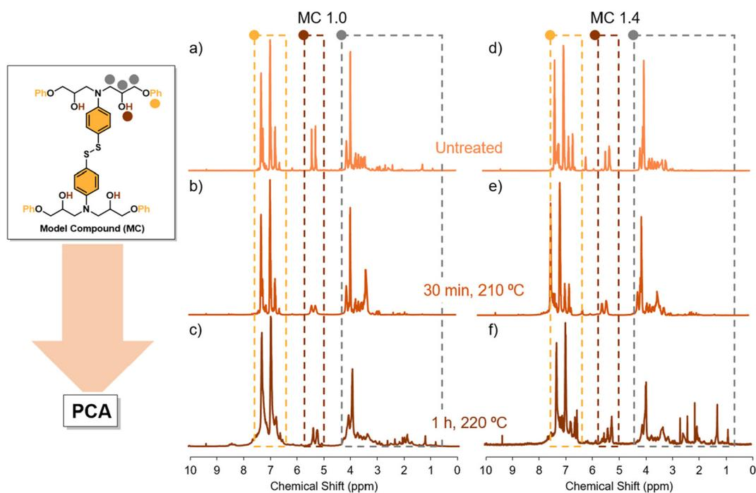
Fig. 3 (a) MC 1.0 spectra without thermal treatment (b) MC 1.0 spectra after being subjected 30 minutes at 210 °C (c) MC 1.0 spectra after 1 hour at 220 °C (d) MC 1.4 spectra without thermal treatment (e) MC 1.4 spectra after being subjected 30 minutes at 210 °C (f) MC 1.4 spectra after 1 hour at 210 °C.
