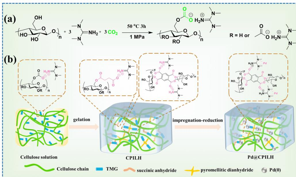
**Fig. 1** The synthesis of CPILH and the Pd@CPILH catalyst. (a) Dissolution of cellulose in the TMG/CO<sub>2</sub>/DMSO solvent system. (b) Schematic diagram of the preparation of CPILH and Pd@CPILH.
