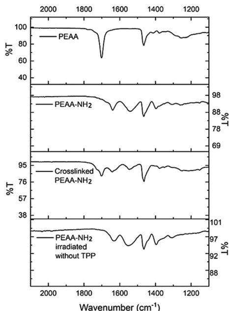
**Fig. 2** A comparison of FTIR spectra of PEEA, PEEA-8C-NH<sub>2</sub>, crosslinked PEEA-8C-NH<sub>2</sub>, and PEEA-8C-NH<sub>2</sub> irradiated without photosensitizer. Similar spectra were observed for PEEA-3C-NH<sub>2</sub>, PEEA-6C-NH<sub>2</sub>, and PEEA-8C-NH<sub>2</sub> between 1100 and 2100 cm<sup>-1</sup>.
