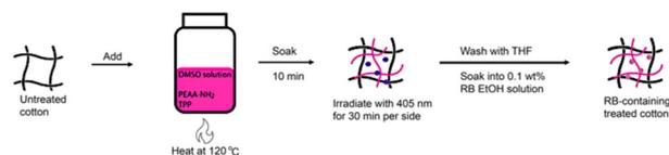
**Fig. 1** Scheme of textile treatment with solution soak and light irradiation resulting in RB-containing PEAA-NH<sub>2</sub> solution-treated cotton.
