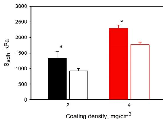
**Fig. 6**  $S_{adh}$  of the adhesives prepared at different coating density in the adhesive joint using p(HEMA-co-SHAM<sub>10</sub>) (filled bars) and p(MEA-co-SHAM<sub>10</sub>) (empty bars). The adhesives were prepared by maintaining a copolymer to PVDF weight ratio of 85 : 15, with an overlapped area of 64.5 mm<sup>2</sup>. \* $p < 0.05$  when compared to MEA-containing adhesive ( $n = 3$ ).
