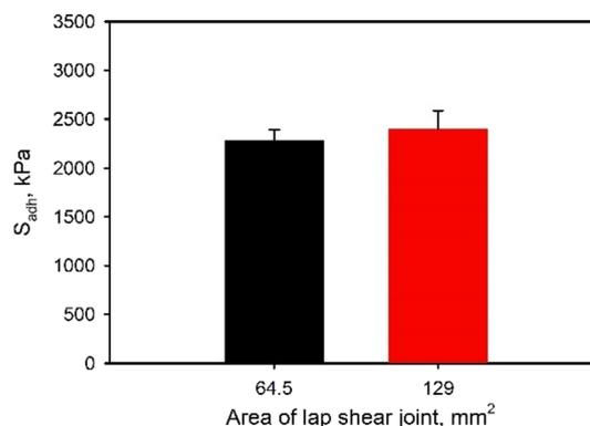
**Fig. 7**  $S_{adh}$  of the adhesives prepared with p(HEMA-co-SHAM<sub>10</sub>) tested with different overlapped area in the adhesive joint. The adhesives were prepared by maintaining a copolymer to PVDF weight ratio of 85 : 15 and a coating density of 4 mg cm<sup>-2</sup> ( $n = 3$ ).
