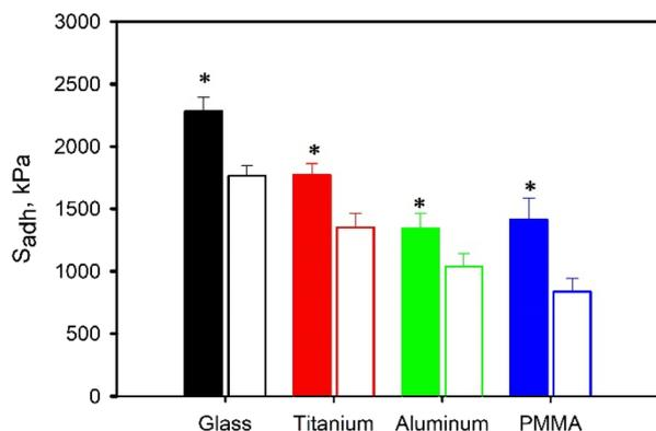
**Fig. 5**  $S_{adh}$  for p(HEMA-co-SHAM<sub>10</sub>) (filled bars) and p(MEA-co-SHAM<sub>10</sub>) (empty bars) tested using different substrates. The adhesives were prepared by maintaining a copolymer to PVDF weight ratio of 85 : 15, with an overlapped area of 64.5 mm<sup>2</sup> and a coating density of 4 mg cm<sup>-2</sup>. \* $p < 0.05$  when compared to MEA-containing adhesive ( $n = 3$ ).
