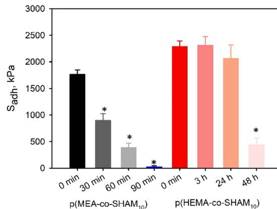
**Fig. 12** Effect of duration of incubation in water on  $S_{adh}$  for adhesive prepared with a copolymer to PVDF weight ratio of 85 : 15, with an overlapped area of 64.5  $\text{mm}^2$  and a coating density of 4  $\text{mg cm}^{-2}$ . \* $p < 0.05$  when compared to the samples tested at time = 0 min ( $n = 3$ ).
