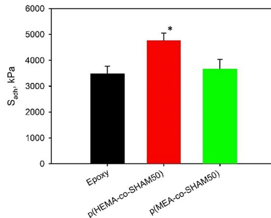
**Fig. 9**  $S_{adh}$  of epoxy, p(HEMA-co-SHAM<sub>50</sub>), and p(MEA-co-SHAM<sub>50</sub>). Adhesive contained a copolymer to PVDF weight ratio of 85 : 15, with an overlapped area of 64.5 mm<sup>2</sup> and a coating density of 4 mg cm<sup>-2</sup>. \* $p < 0.05$  when compared to epoxy ( $n = 3$ ).
