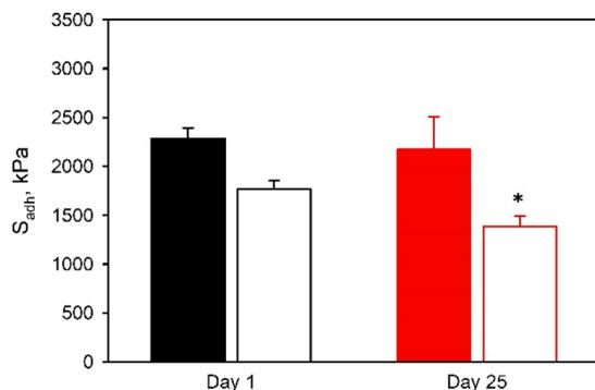
**Fig. 11** 25-Day aging analysis of adhesively bonded samples exposed to open air (temperature  $\approx 21.5$  °C, humidity  $\approx 20\%$ ). The adhesive was prepared using p(HEMA-co-SHAM<sub>10</sub>) (filled bars) and p(MEA-co-SHAM<sub>10</sub>) (empty bars) a copolymer to PVDF weight ratio of 85 : 15, with an overlapped area of 64.5  $\text{mm}^2$  and a coating density of 4  $\text{mg cm}^{-2}$ . \* $p < 0.05$  when compared to the same adhesive formulation tested at Day 1 ( $n = 3$ ).
