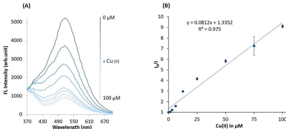
**Fig. 8** Concentration-dependent fluorescence quenching via Cu(II) on HisBD. (A) Decrease of fluorescence via an increase of added Cu(II) on HisBD (100  $\mu\text{M}$ ). (B) Fluorescence intensity changes of HisBD (in  $I_0/I$ ) by Cu(II) concentration.  $I_0$  represents the starting fluorescence intensity of HisBD (100  $\mu\text{M}$ ), and  $I$  the fluorescence intensity after the addition of Cu(II). Data represented as mean  $\pm$  SD: ( $n = 3$ ).
