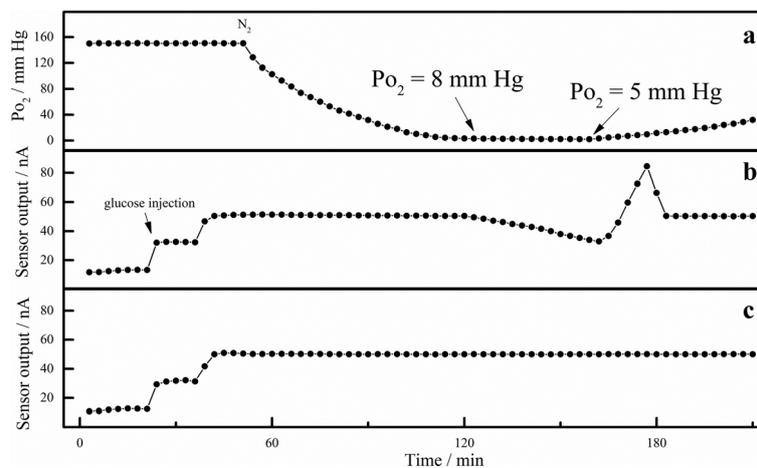
**Fig. 2** The oxygen effect of PDMS/HT blending membrane modified CGM sensor with different PDMS content, (a)  $PO_2$  in the system; (b) PDMS/HT with a weight ratio of 5 : 50 modified CGM sensors; (c) PDMS/HT with a weight ratio of 10 : 50 modified CGM sensors.
