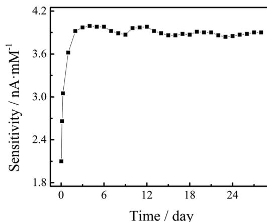
**Fig. 3** The stability test of PDMS/HT modified glucose sensors in PBS solution (pH 7.4, with different glucose concentrations from 0, 5.0, 10.0, 15.0, 20.0, 25.0, and 30.0 mM) at  $32.0 \pm 0.5 \text{ }^\circ\text{C}$  during 28 days. The stability was deemed as the sensitivity variations, and the sensitivity was calculated according to the slope of the current of the glucose sensors and glucose concentrations.
