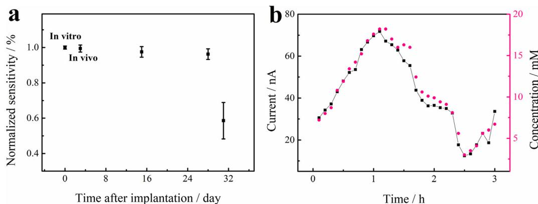
**Fig. 6** (a) Sensitivity *in vivo* of glucose sensors for 31 days. The data are the means of measurements from 9 sensors. Error bars are  $\pm$  SD. (b) Interstitial glucose concentrations (solid line) were obtained for one representative sensor during glycemic clamp procedures, and corresponding blood glucose concentrations (red circles) were concurrently measured using a veterinary glucometer method. Notice the lag between changes in blood glucose concentrations and CGMS values.
