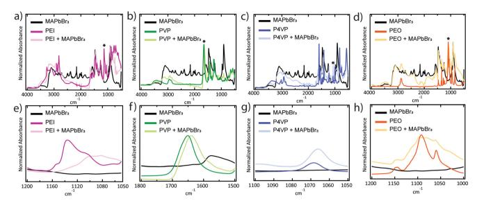
Fig. 6 FTIR spectra of composite materials and individual perovskite and polymer components. Spectra of neat MAPbBr<sub>3</sub> samples compared to FTIR spectra of neat polymers PEI, PVP, P4VP, and PEO, and the corresponding perovskite/polymer composite samples. (a–d) Show the full spectra where (e–h) are in a narrow range to highlight peaks of interest for the C–N stretch in PEI, the C=O stretch in PVP, the C–N stretch in P4VP, and the C–O stretch in PEO.
