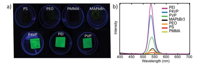
Fig. 3 Emission fluorimetry of perovskite/polymer films under 365 nm excitation. (a) Photographs of photoluminescent perovskite/polymer films on glass irradiated with a 365 nm UV lamp. MAPbBr<sub>3</sub> is the pure perovskite material prepared by the precipitation method without polymer. (b) Fluorescence emission spectra of perovskite/polymer films excited with 365 nm wavelength.
