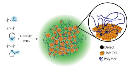
Fig. 7 Schematic of polymer macroligand encapsulation of perovskite nanocrystals. The prediction is such that nitrogen-containing polymers will strongly bind to the crystal surface, passivating the trap sites that form during synthesis.
