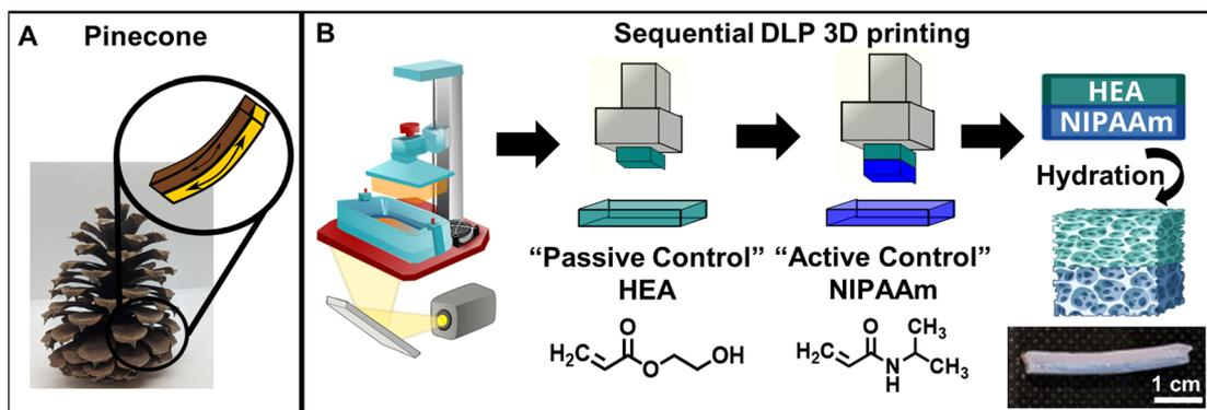
**Fig. 1** Fabrication of bilayer hydrogels using sequential DLP 3D printing. A. Natural inspiration from pinecone bilayer structure. B. Overall schematic for fabrication of monolayer and bilayer hydrogels using DLP printing.
