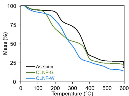
**Fig. 2** TGA thermograms of coaxially electrospun *L. lactis* into alginate-based nanofibers also containing CaCO<sub>3</sub> as as-spun (solid, black line), CLNF-W (solid, blue line), and CLNF-G (solid, green line) nanofiber samples.
