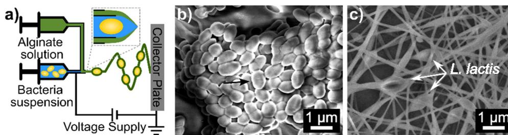
**Fig. 1** Schematic (a) of coaxial electrospinning for the encapsulation of bacteria in alginate-based nanofibers. (b) Unencapsulated *L. lactis* and (c) alginate-based nanofibers with encapsulated *L. lactis* that were coaxially electrospun using a 0.35/0.70 mL h<sup>-1</sup> core/shell flow rate. Other electrospinning conditions are listed in the methods section. The arrow indicates the location of an *L. lactis* cell.
