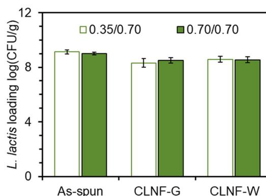
**Fig. 3** *L. lactis* loading of coaxially electrospun *L. lactis* into alginate-based nanofibers containing antacid before (as-spun) and after crosslinking (CLNF-G and CLNF-W) using 0.35/0.70 (green outline, white fill) and 0.70/0.70 mL h<sup>-1</sup> (black outline, green fill) core/shell flow rates. Other electrospinning conditions are reported in the Methods Section. All values are statistically equivalent. ( $n = 3$ ;  $p < 0.05$ ).
