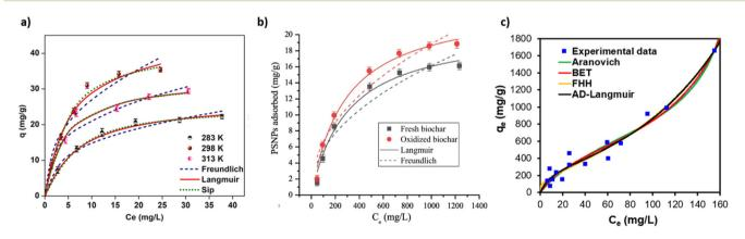
Fig. 10 Adsorption isotherm curves of (a) PS NPs onto sugarcane Bagasse biochar at varying adsorption temperatures. Adapted from ref. 200 with permission from Elsevier. Copyright ©2021; (b) PS NPs onto oxidized and non-oxidized corncob biochar. Adapted from ref. 201 with permission from Elsevier. Copyright ©2021; and (c) PET NPs onto epoxy AC. Adapted from ref. 110 with permission from Elsevier. Copyright ©2023.
