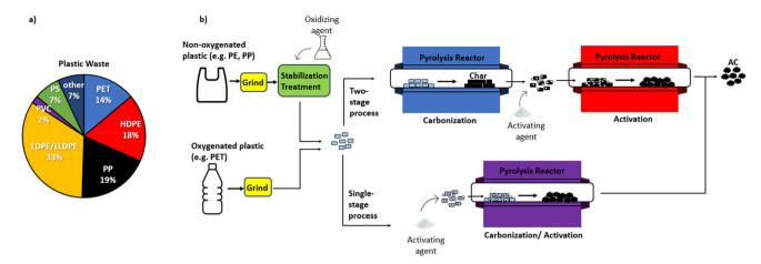
Fig. 6 (a) Composition of plastic waste managed in the US in 2019. Data obtained from ref. 11; (b) illustration of various pathways for the chemical activation of oxygenated and non-oxygenated plastics.
