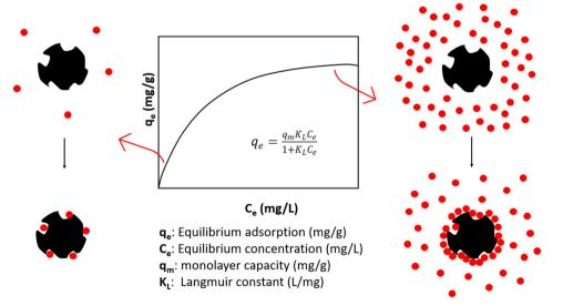
Fig. 7 Langmuir adsorption isotherm and corresponding illustrations of adsorption onto AC at low and high solute concentrations. 187
