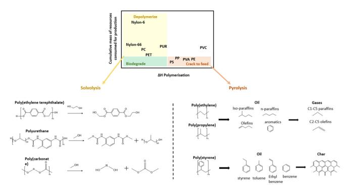
Fig. 2 (a) Mapping of the recommended chemical recycling technique for different plastics;<sup>14</sup> (b) schematic of the glycolysis of PET and methanolysis of PUR and PC; (c) general pyrolysis products of PE, PP and PS.
