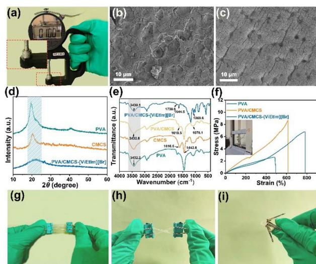
**Fig. 2** (a) The thickness test of the PVA/CMCS-[ViEtIm][Br] hydrogel (the inset is the photo of the tested hydrogel), SEM images of (b) PVA/CMCS gel and (c) PVA/CMCS-[ViEtIm][Br] gel, (d) XRD patterns and (e) FT-IR images of PVA, CMCS, PVA/CMCS and PVA/CMCS-[ViEtIm][Br], (f) the stress-strain curves of PVA, PVA/CMCS and PVA/CMCS-[ViEtIm][Br] hydrogels, and (g-i) twisting and bending of the PVA/CMCS-[ViEtIm][Br] hydrogel.
