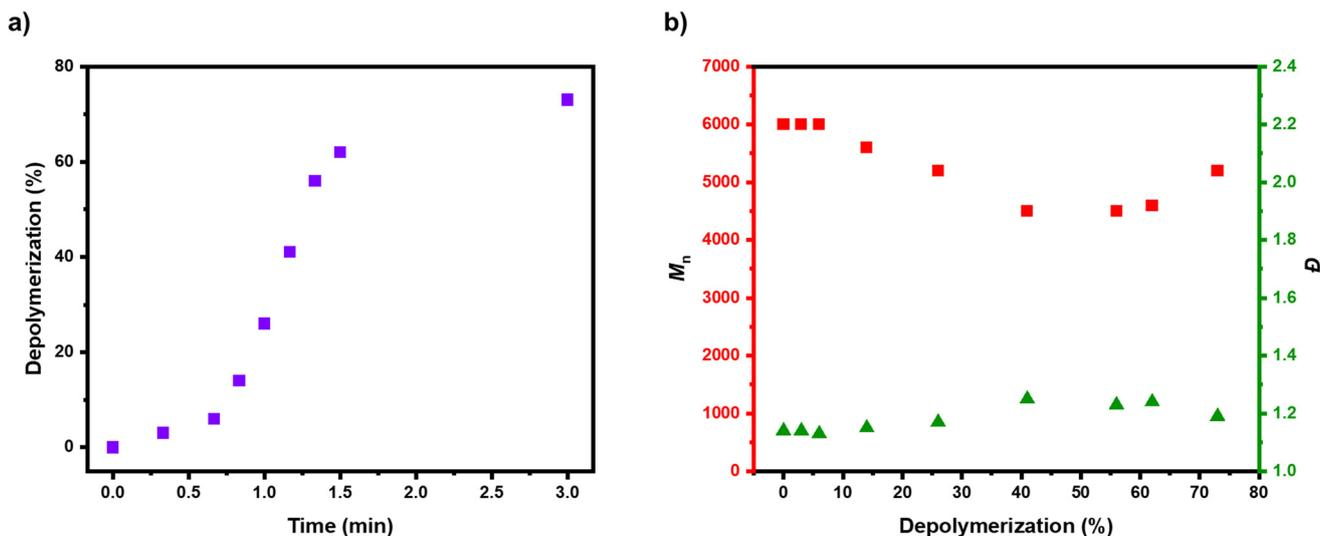
Fig. 4 Depolymerization kinetics with the optimized conditions ([P-Br]:[FeBr<sub>2</sub>]:[TBABr] of 1:1:1). In (a) the evolution of depolymerization conversion with time is shown and in (b) the evolution of molecular weight and dispersity with depolymerization is presented.
