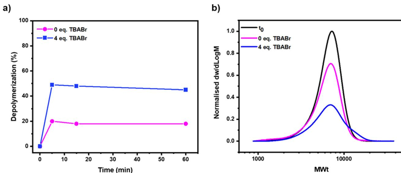
**Fig. 1** The effect of TBABr on the depolymerization of bromine-terminated polymers synthesized by ATRP. In (a) kinetics illustrate the depolymerization conversion obtained from  $^1\text{H}$  NMR and in (b) SEC traces under the various conditions are illustrated after 60 minutes of depolymerization. Both reactions were performed with a 50 mM repeat unit concentration of polymer at 170 °C in TEGDME.
