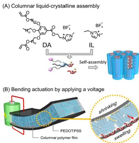
**Fig. 15** (A) Molecular structures of the wedge-shaped imidazolium compound with diacrylate groups (DA) and ionic liquid [EMIM][BF<sub>4</sub>] (IL) and their self-assembly into the columnar liquid-crystalline phase forming 1D ion channels. (B) Illustration of the electric-field-driven bending actuation of the three-layer membranes composed of the columnar liquid crystalline polymer electrolyte and PEDOT:PSS electrodes. Reproduced from ref. 107 with permission from ACS, Copyright [2022].
