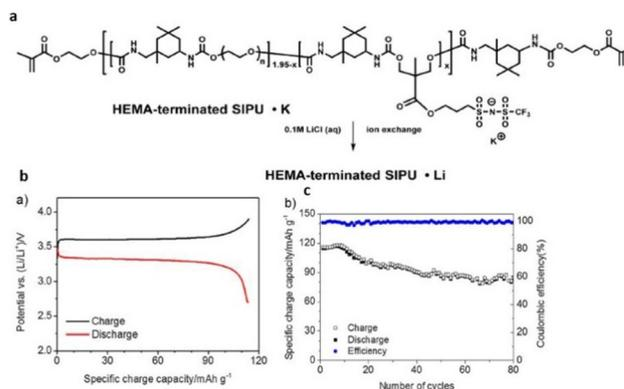
**Fig. 31** (a) Schematic representation of the polyurethane-based polymer investigated in the current study. (b) Lithium metal/XSIPU-PC/LiFePO<sub>4</sub> cell potential versus specific discharge capacity at  $C/10$  and ambient temperature; (c) specific capacity versus cycle number. Reproduced from ref. 211 with permission from Elsevier, Copyright [2017].
