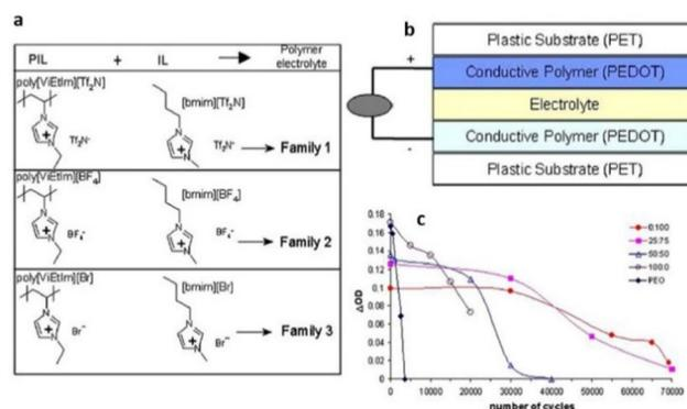
**Fig. 28** (a) Composition of the polymer electrolyte families. (b) All-polymeric five-layer electrochromic device configuration. (c) Variation of DOD as a function of the number of cycles for ECDs using polymer electrolytes with different ratios [EMIM][Br]: poly[ViEtm][Br] and using PEO/lithium triflate electrolyte. Reproduced from ref. 179 with permission from Elsevier, Copyright [2006].
