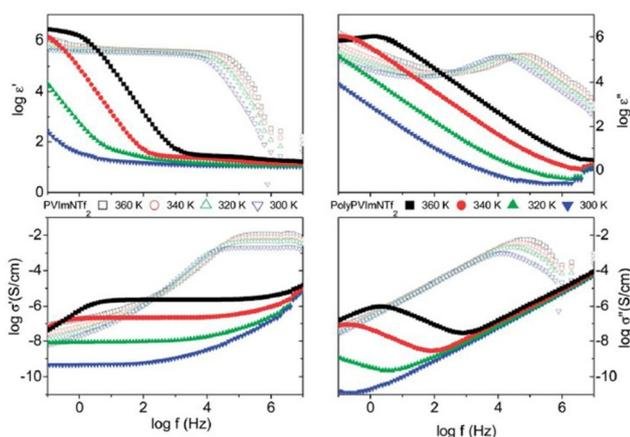
**Fig. 22** The complex dielectric function  $\epsilon^*(\epsilon' - i\epsilon'')$  and the complex conductivity function  $\sigma^*(\sigma' + i\sigma'')$  versus frequency at different temperatures as indicated for the polymerized ionic liquid (poly(PVIM) NTf<sub>2</sub>) (closed symbols) and the corresponding low molecular weight ionic liquid (open symbols) at selected temperatures. Reproduced from ref. 20 with permission from RSC, Copyright [2014].
