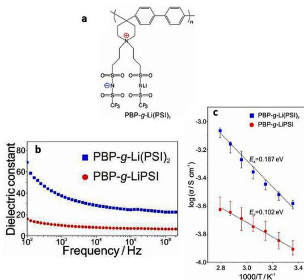
**Fig. 60** (a) Schematic representation of grafted poly(biphenyl piperidinium)s including PBP-g-Li(PSI)<sub>2</sub> (b) dielectric spectra of PBP-g-Li(PSI)<sub>2</sub> and PBP-g-LiPSI (c) ionic conductivity of PBP-g-LiPSI and PBP-g-Li(PSI)<sub>2</sub> gel blend polymer electrolyte membranes. Reproduced from ref. 247 with permission from Elsevier, Copyright [2022].
