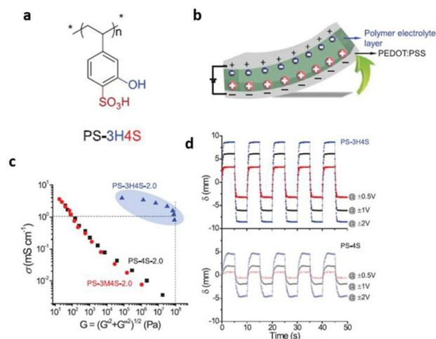
**Fig. 13** (a) Schematic representation of PS-3H4S polymer used in the study. (b) Schematic illustration depicting bending deformation of ionic polymer actuators under an applied voltage. (c) Conductivity–modulus relationship of PS-3H4S-2.0, PS-3M4S-2.0, and PS-4S-2.0. (d) Bending displacements of PS-3H4S actuator at ±0.5, ±1 and ±2 V, compared with PS-4S counterparts. Reproduced from ref. 93 with permission from Wiley-VCH, Copyright [2022].
