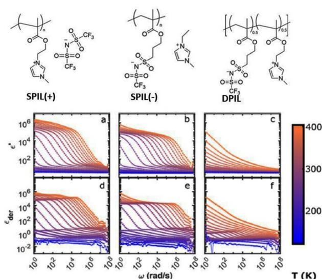
**Fig. 67** Schematic representation of the polymers investigated in the study. Frequency dependence of (a–c) the dielectric permittivity and (d–f) the dielectric loss derivative  $\epsilon'_{\text{der}}$  for (a and d) SPIL(+), (b and e) SPIL(–), and (c and f) DPIL across the range of temperatures investigated in the study. Reproduced from ref. 22 with permission from ACS, Copyright [2021].
