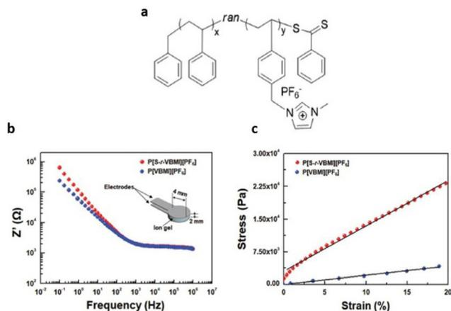
**Fig. 26** (a) Schematic representation of the random copolymer-based ion-conductive gel. (b) Resistance ( $Z'$ ) versus frequency (Hz) plots and (c) stress–strain curves for the ion gels composed of 40 wt% P[S-*r*-VBMI][PF<sub>6</sub>] or P[VBMI][PF<sub>6</sub>] and 60 wt% [EMIM][TFSI]. The inset of (b) depicts the electrode/ion gel/electrode cell structure used in electrochemical impedance spectroscopy (EIS) experiments. Reproduced from ref. 4 with permission from Wiley-VCH, Copyright [2018].
