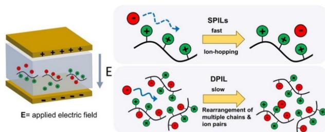
**Fig. 68** Schematic illustration of the bulk ion transport in DPILs vs. SPILs. In SPILs, individual ions can move relatively independently of other charged units. However, in DPILs movement of a single ion requires rearrangement of multiple chains and ion pairs. Reproduced from ref. 22 with permission from ACS, Copyright [2021].
