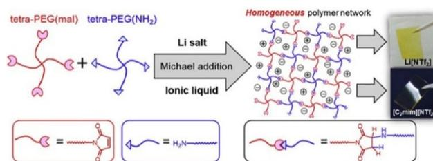
Fig. 24 Formation of polymer electrolytes with a homogeneous PEG network via Michael addition reaction and containing either Li[N(Tf<sub>2</sub>)] or [C<sub>2</sub>mim][NTf<sub>2</sub>]. Reproduced from ref. 204 with permission from Elsevier, Copyright [2019].
