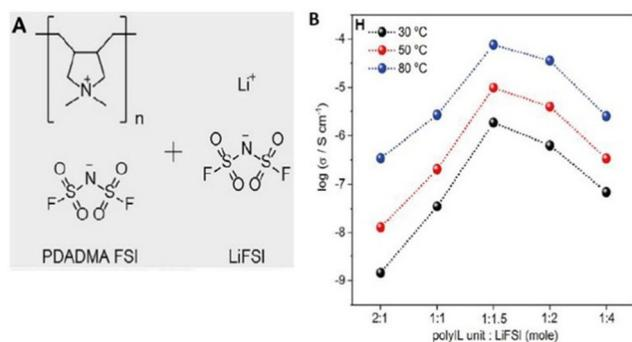
**Fig. 34** (A) The chemical structures of poly(diallyldimethylammonium) bis(fluorosulfonyl)imide (PDADMA FSI) and Li bis(fluorosulfonyl)imide (LiFSI) salt. (B) The ion conductivities of different poly/L systems at 30 °C, 50 °C, and 80 °C, respectively. The highest conductivity of  $0.7 \times 10^4 \text{ S cm}^{-1}$  is achieved for the 1 : 1.5 system at 80 °C. Reproduced from ref. 214 with permission from Elsevier, Copyright [2019].
