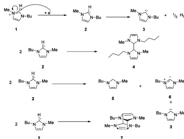
**Fig. 2** Reduction of  $[\text{C}_4\text{mim}]^+$  cation 1 through radical and carbene formation followed by dimer formation or disproportionation, or cage-like structure formation of the  $[\text{C}_4\text{mim}]^+$  radical. Reproduced from ref. 37 with permission from ACS, Copyright [2005].
