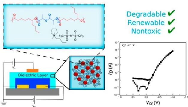
**Fig. 8** Schematic representation of a degradable and biocompatible ion gels from a renewable ABA triblock polyester and ionic liquid. Reproduced from ref. 73 with permission from ACS, Copyright [2017].
