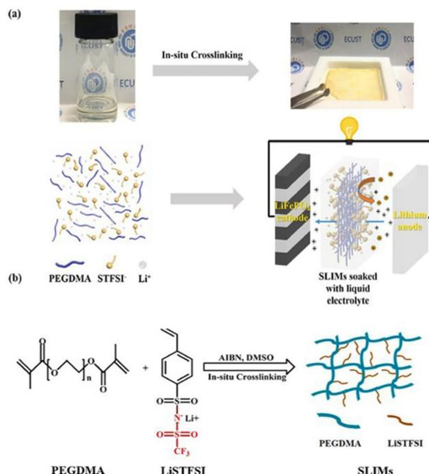
**Fig. 36** (a) The images of the precursor solution and SLIMs after *in situ* crosslinking, with the corresponding change of structures. (b) Preparation process of SLIMs by *in situ* crosslinking reaction. Reproduced from ref. 216 with permission from Elsevier, Copyright [2020].
