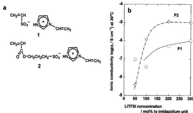
**Fig. 62** (a) Structure of ionic liquid monomers obtained by neutralization. (b) Effect of LiTFSI concentration on the ionic conductivity of corresponding polymers P1 and P2. Reproduced from ref. 23 with permission from Wiley-VCH, Copyright [2002].
