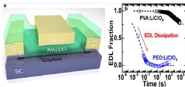
**Fig. 65** (a) Schematic representation of the graphene FET fabricated; (b) enhancing the room-temperature electric double layer retention time in 2-D crystal FETs. Reproduced from ref. 251 with permission from ACS, Copyright [2017].
