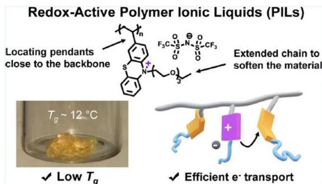
**Fig. 53** Schematic structure of redox polymers with tethered chains inserted in between the backbone and pendants to target for low  $T_g$  charge conducting polymers. Reproduced from ref. 233 with permission from ACS, Copyright [2021].
