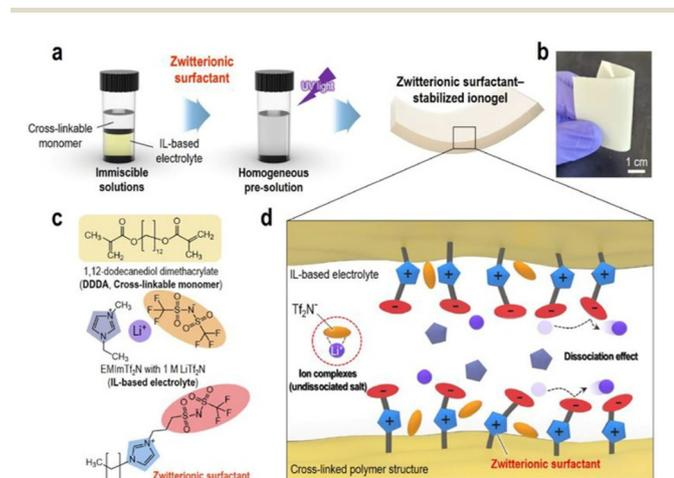
**Fig. 11** (a) Schematic preparation and (b) representative photograph of zwitterionic surfactant-stabilized ionogels. (c) Chemical structures of pre-solution components. (d) Schematic of ion-dipole interactions within zwitterionic surfactant-stabilized ionogel electrolytes. Reproduced from ref. 80 with permission from Elsevier, Copyright [2023].
