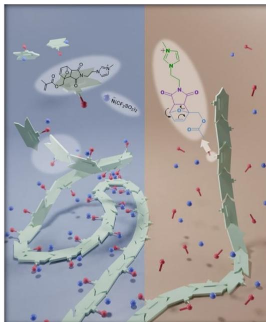
**Fig. 52** Schematic illustration of temperature-dependent ion release in polymerized ionic liquids containing thermally labile Diels–Alder linkages. Reproduced from ref. 15 with permission from ACS, Copyright [2020].
