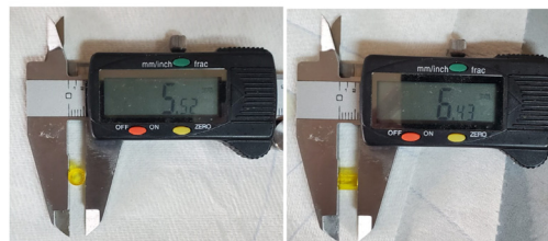
Fig. 1 Design of the 3D printing hydrogels used in the 96 well plate analysis. ( H = 7 mm, R = 5.4 mm, r = 3.6 mm), and a sample of the printed model with measured dimensions.
