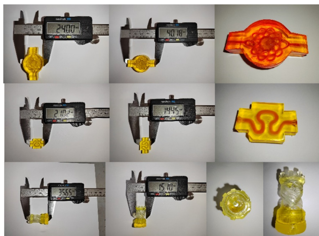
Fig. 15 Examples of DLP-printed objects with internal channels or a refined geometry demonstrating their capability for fabricating high resolution objects.
