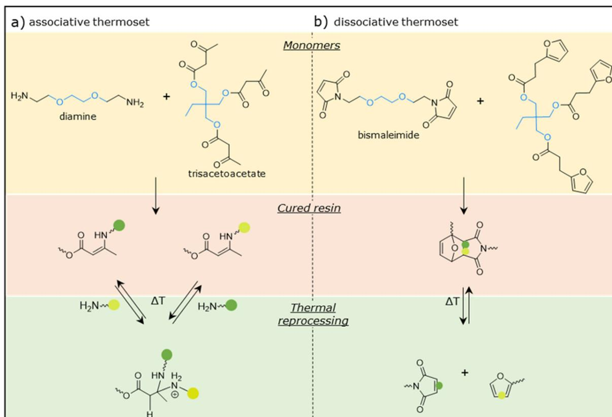
**Fig. 2** (a) Synthesis of the associative thermoset based on a diamine and trisacetoacetate yielding a resin with vinylogous urethane linkages. (b) Synthesis of the dissociative thermoset based on bismaleimide and trifuran yielding a resin with DA linkages. The respective reversible mechanisms responsible for the thermal reprocessability are depicted at the bottom.
