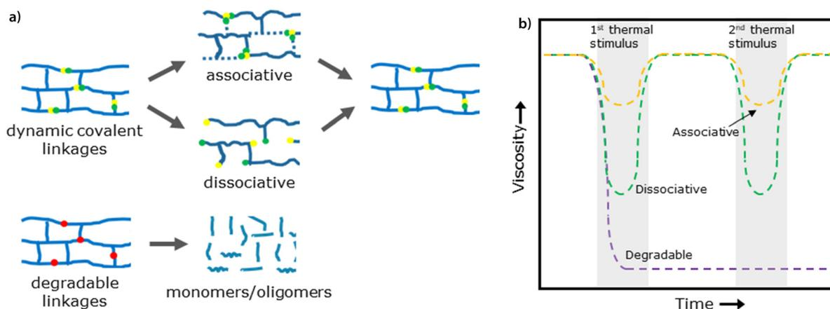
**Fig. 1** (a) Schematic representation of associative, dissociative and degradable linkages in a thermoset network when applying a thermal stimulus. Only dissociative and associative linkages can reform a cross-linked network, whereas degradable linkages will result in the formation of monomers or oligomers. (b) Graphical representation of the theoretical viscosity as a function of time when applying a thermal stimulus to associative, dissociative and degradable linkages.
