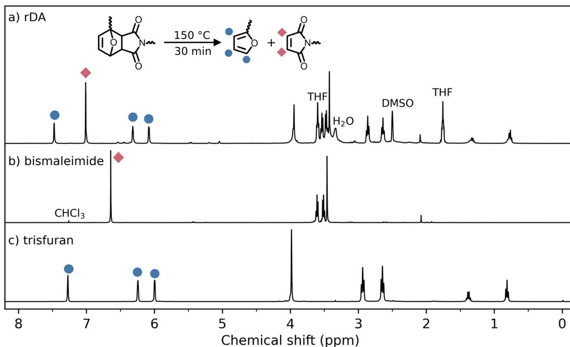
Fig. 5 <sup>1</sup>H-NMR spectra of (a) the DA-adduct after 30 minutes at 150 °C in DMSO-*d*<sub>6</sub>, (b) the bismaleimide monomer recorded in CDCl<sub>3</sub> and (c) the trisfuran monomer recorded in CDCl<sub>3</sub>. The THF observed in spectrum (a) is attributed to residual THF after the swelling tests.
