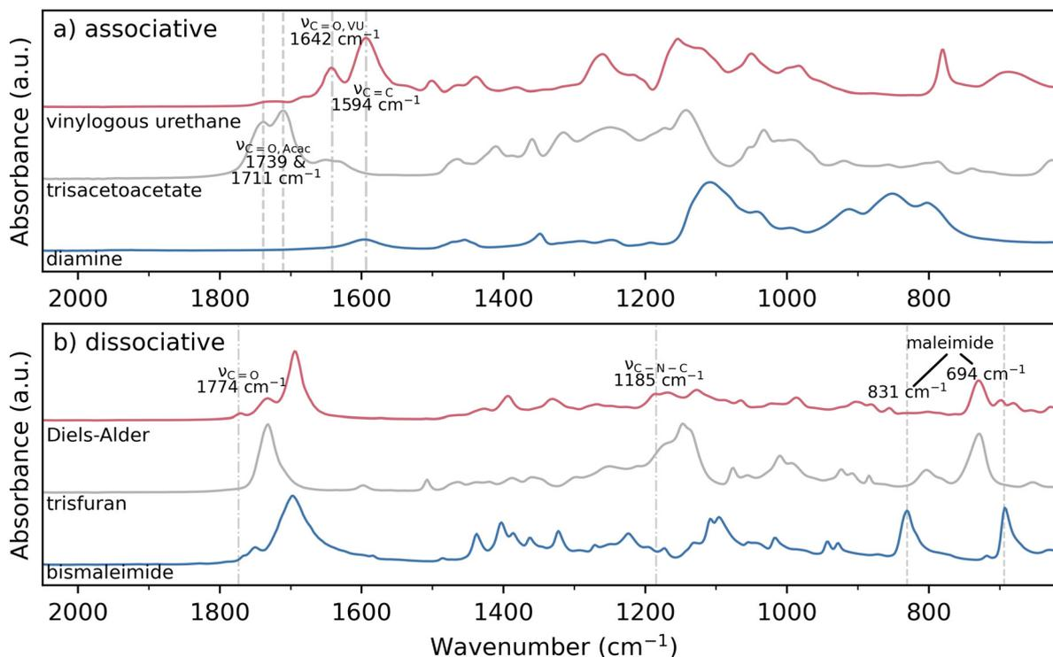
**Fig. 3** Magnified ATR-FTIR spectra of the monomers and the cured thermosets recorded at room temperature. (a) Trisacetoacetate and the cured vinyllogous urethane thermoset. (b) Bismaleimide, trisfuran, and the cured DA thermoset. The full scale spectra can be found in ESI Fig. S2.†
