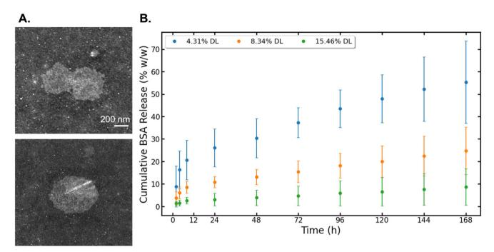
Fig. 6 (A) STEM images of 8.34% DL BSA-BCNPs/P80. Scale bar set to 200 nm. (B) Results for cumulative BSA drug release (% w/w) from BCNPs/ P80, calculated using egn (6).
