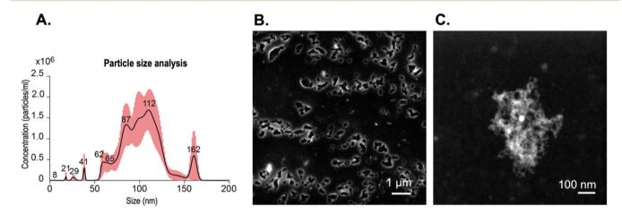
Fig. 5 (A) Hydrodynamic size of BCNPs at concentration of  $8.35 \times 10^7 \pm 1.18 \times 10^7$  particles mL<sup>-1</sup> and measured on nanoparticle tracking analysis. The red region indicates peak intensity and standard deviation; (B) STEM of BCNPs at 1 µm scale bar, and (C) STEM of a BCNP at 100 nm scale bar.
