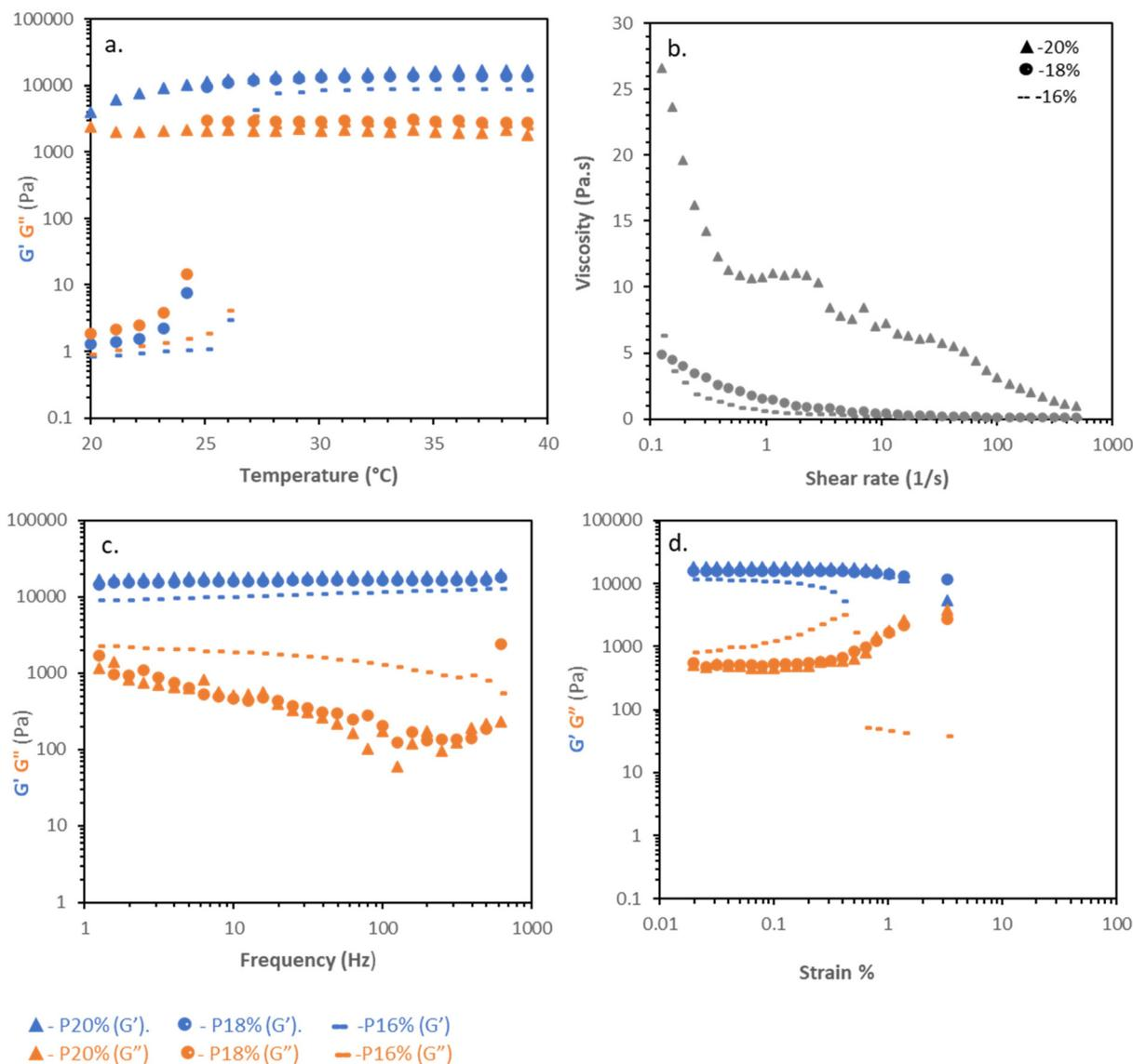
**Fig. 2** Rheological properties of Poloxamer407(P) solutions at concentrations 16%, 18% and 20% (w/v) in CCM: (a) temperature ramps at a fixed strain (0.1%) and frequency (6.283 rad per s). (b) Flow rheology at 20 °C. (c) frequency sweeps at 0.1% strain and 37 °C. (d) Amplitude sweeps at 6.283 rad per s and 37 °C.
