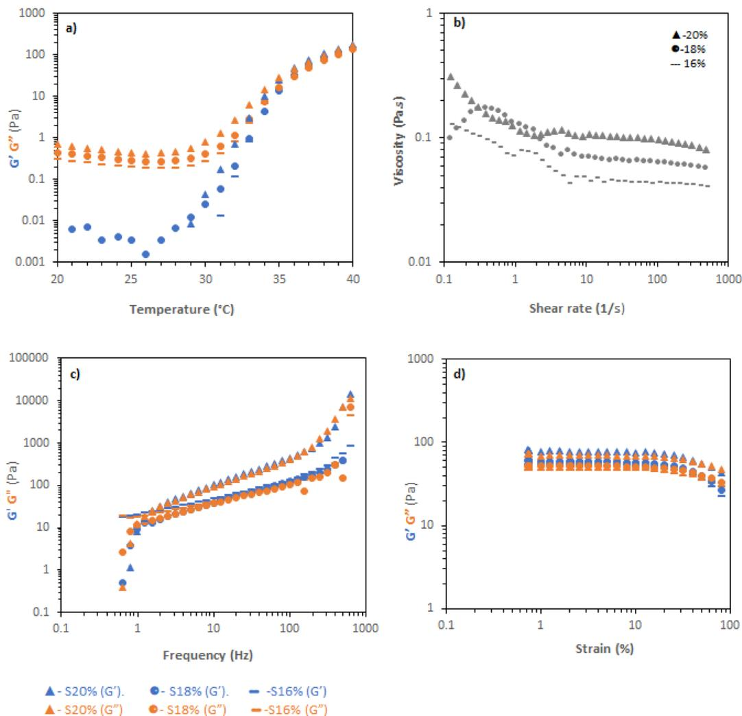
**Fig. 3** Rheological properties of Soluplus(S) solutions at concentrations 18% and 20% (w/v): (a) temperature ramps at a fixed strain (0.1%) and frequency (6.283 rad per s). (b) Flow rheology at 20 °C. (c) frequency sweeps at 0.1% strain and 37 °C. (d) Amplitude sweeps at 6.283 rad per s and 37 °C.
