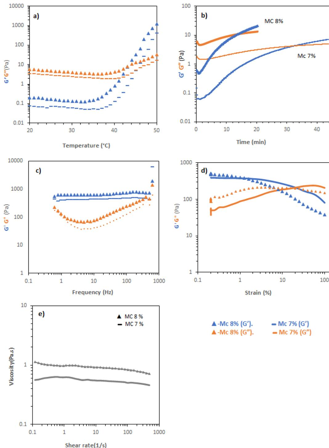
**Fig. 4** Rheological properties of MC at concentration 7% and 8% w/v (MC 7% and MC 8%, respectively): (a) temperature ramps at a fixed strain (0.1%) and frequency (6.283 rad per s). (b) Time-dependence of rheological response (0.1% strain, 6.283 rad per s) at 37 °C. (c) Frequency sweeps at 0.1% strain and 37 °C. (d) Amplitude sweeps at 6.283 rad per s and 37 °C. (e) Flow rheology at 20 °C.
