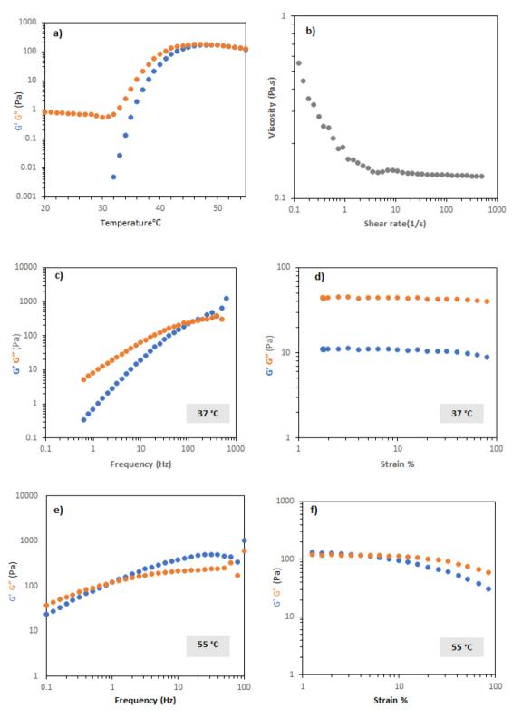
Fig. 5 Rheological properties of PNIPAM-b-PEO-b-PNIPAM solution at concentration 20% (w/v): (a) temperature ramps at a fixed strain (0.1%) and frequency (6.283 rad per s). (b) Flow rheology at 20 °C. (c) Frequency sweeps at 0.1% strain and 37 °C. (d) Amplitude sweeps at 6.283 rad per s and 37 °C. (e) Frequency sweeps at 0.1% strain and 55 °C. (f) Amplitude sweeps at 6.283 rad per s and 55 °C.
