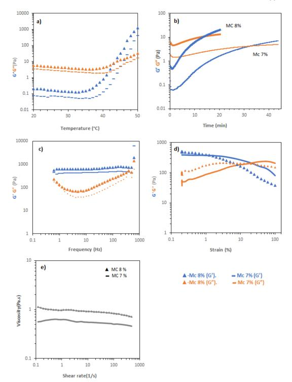
Fig. 4 Rheological properties of MC at concentration 7% and 8% w/v (MC 7% and MC 8%, respectively): (a) temperature ramps at a fixed strain (0.1%) and frequency (6.283 rad per s). (b) Time-dependence of rheological response (0.1% strain, 6.283 rad per s) at 37 °C. (c) Frequency sweeps at 0.1% strain and 37 °C. (d) Amplitude sweeps at 6.283 rad per s and 37 °C. (e) Flow rheology at 20 °C.
