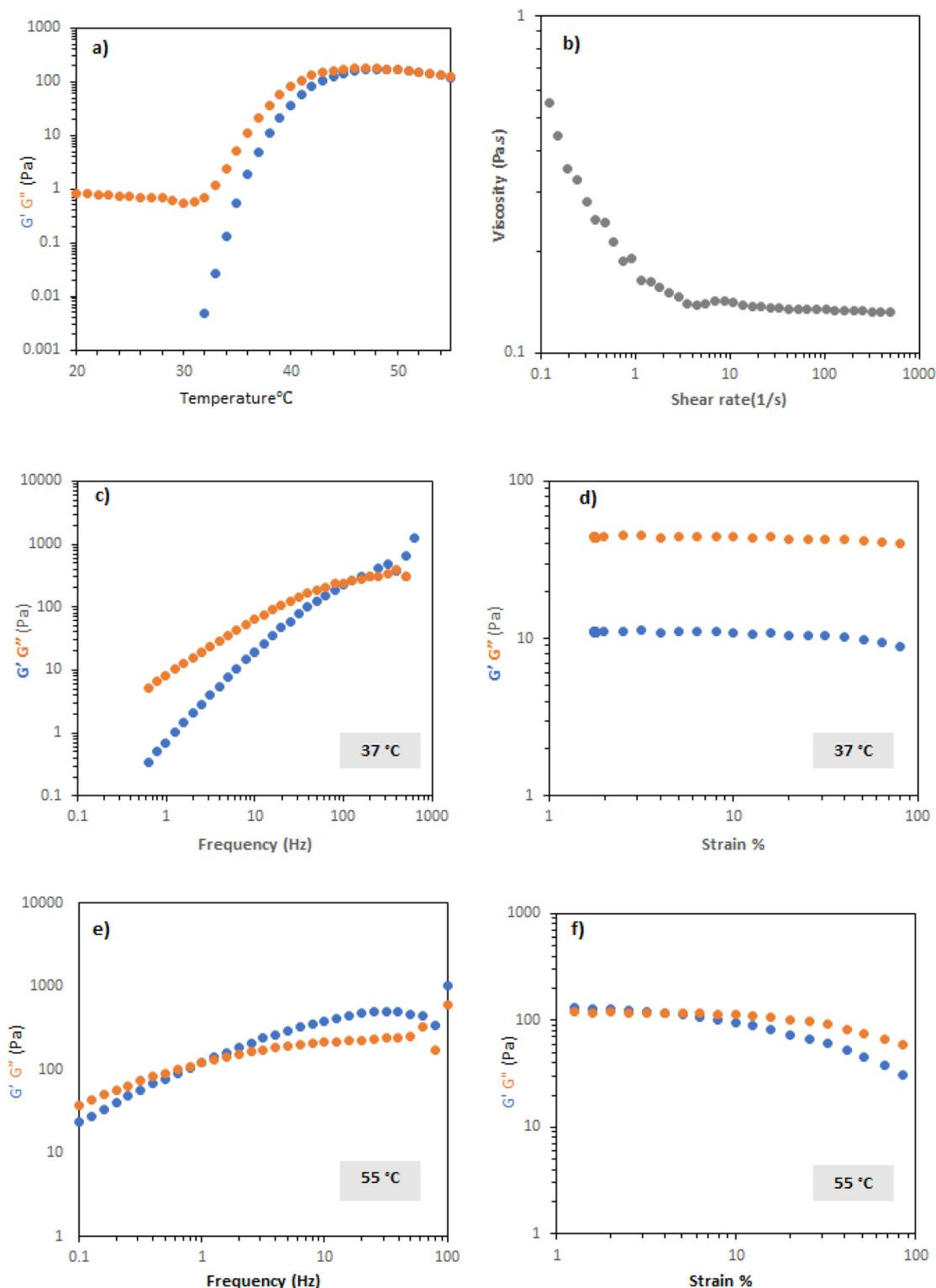
**Fig. 5** Rheological properties of PNIPAM-*b*-PEO-*b*-PNIPAM solution at concentration 20% (w/v): (a) temperature ramps at a fixed strain (0.1%) and frequency (6.283 rad per s). (b) Flow rheology at 20 °C. (c) Frequency sweeps at 0.1% strain and 37 °C. (d) Amplitude sweeps at 6.283 rad per s and 37 °C. (e) Frequency sweeps at 0.1% strain and 55 °C. (f) Amplitude sweeps at 6.283 rad per s and 55 °C.
