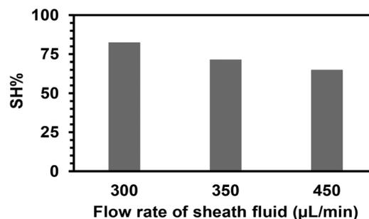
**Fig. 5** Efficiency of the covalent attachment of (SH)<sub>3</sub> on the microfibers relative to the quantity used in the sheath phase for different flow rates of the sheath phase.
