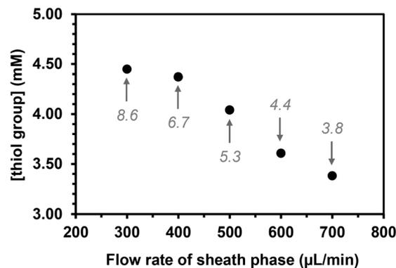
**Fig. 4** Effect of the flow rate of the sheath phase (10 mol% (SH)<sub>3</sub>) on the quantity of free thiol groups present at the surface of PEGDA microfibers (flow rate of the core phase = 2 μL min<sup>-1</sup>). The values in italics are the average time in seconds for a molecule present in the core phase to travel from the capillary exit to the end of the UV arrangement.
