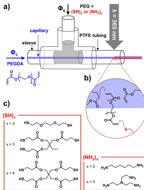
**Fig. 1** Simultaneous production of polymer microfibers by photopolymerization and their surface modification with thiol or amine groups: (a) capillary-based microfluidic device used with (b) highlight of the reactions occurring at the interface of the two phases (illustrated with molecules with thiol groups) and (c) the structure of molecules with multiple thiols and amines used.
