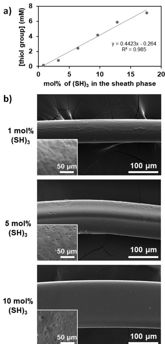
**Fig. 3** Effect of the concentration of (SH)<sub>3</sub> used in the sheath phase on (a) the quantity of free thiol groups at the surface of PEGDA microfibers as determined by Ellman's test (fiber mass = 10 mg, flow rate of the sheath phase = 350 μL min<sup>-1</sup>, flow rate of the core phase = 1.5 μL min<sup>-1</sup>) and (b) the surface integrity of the microfibers imaged by SEM with a zoom at higher magnification on the fiber surface to show its texture in the insets.
