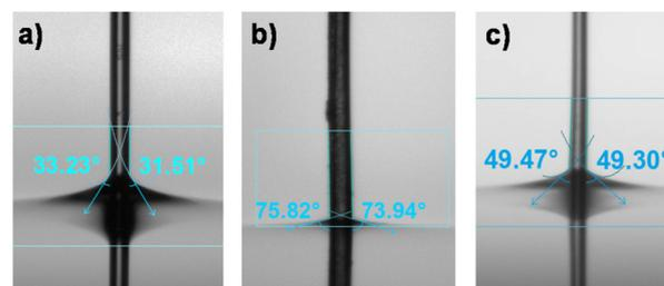
Fig. 7 Contact angle measurement of PEGDA microfibers using the Wilhelmy method for the (a) unmodified, (b)  $(\text{SH})_3$ -modified, and (c)  $(\text{NH}_2)_3$ -modified microfibers. The fibers were prepared using the following conditions:  $Q_s = 350 \mu\text{L min}^{-1}$ ,  $Q_c = 1.5 \mu\text{L min}^{-1}$ , concentration of  $(\text{SH})_3$  and  $(\text{NH}_2)_3$  in the sheath phase = 10 mol%.
