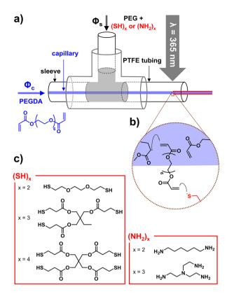
Fig. 1 Simultaneous production of polymer microfibers by photopolymerization and their surface modification with thiol or amine groups: (a) capillary-based microfluidic device used with (b) highlight of the reactions occurring at the interface of the two phases (illustrated with molecules with thiol groups) and (c) the structure of molecules with multiple thiols and amines used.
