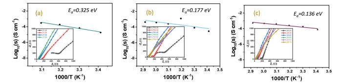
**Fig. S2** Arrhenius plot of conductivity  $\nu$ s. 1/Temperature for the three different pellet compositions: (a) LP, (b) LPM, (c) LM. The insets show the corresponding Nyquist plots at different temperatures.
