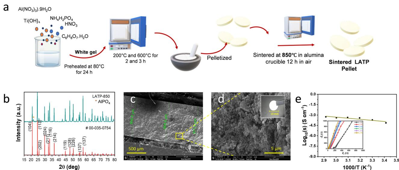
**Fig. 1** (a) Schematic representation of the synthesis of LAMP pellets. (b) XRD patterns, (c) cross-section SEM image, and (d) SEM image of an LAMP pellet. Inset of (d) shows a digital photograph of the pellet. (e) Ionic conductivity plot of LAMP.
