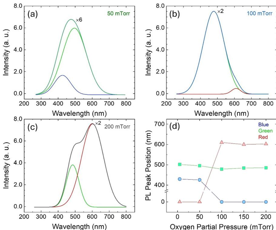
Fig. 8 (a–c) Room temperature PL spectroscopy of the W-incorporated  $\beta$ -Ga<sub>2</sub>O<sub>3</sub> films. (d) PL peak position as a function of  $pO_2$ .
