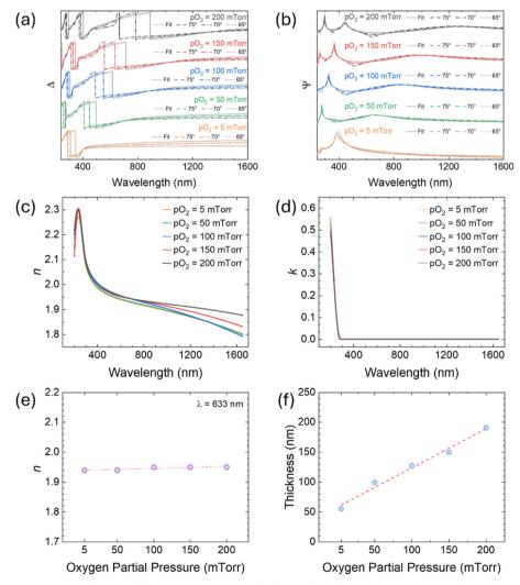
Fig. 6 SE data of as-grown samples. (a and b) Representative plots of psi and delta functions extracted at different angles of incidence of the sample grown at varying pO2. (c and d) Refractive index and extinction coefficient of all the samples. (e and f) Refractive index at a wavelength of 633 nm and pressure-dependent thickness variation of all the samples.
