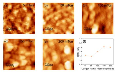
Fig. 4 AFM data of PLD GWO films deposited at varying pO<sub>2</sub>. (a-e) AFM surface morphology scans; and (f) RMS roughness variation with pO<sub>2</sub> for PLD GWO films. The effect of  $pO_2$  on the morphology and roughness of PLD GWO films is evident.
