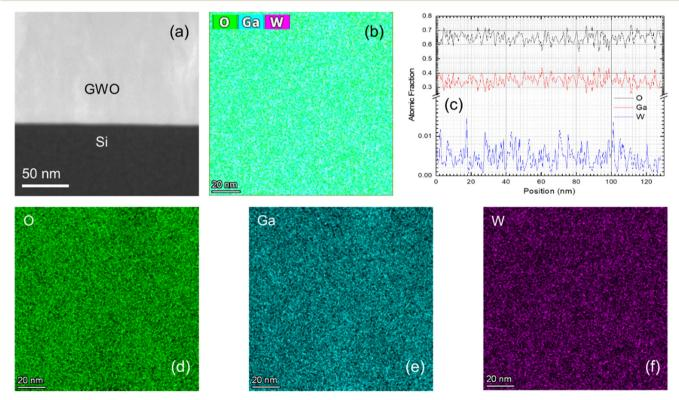
Fig. 5 Cross sectional TEM images: (a) high-resolution HAADF STEM images of W-incorporated  $\beta$ -Ga<sub>2</sub>O<sub>3</sub> films on a Si platform. (b and c) Elemental color mapping and corresponding atomic fraction plots for Ga, O, and W, respectively. (d-f) Individual color mapping of O, Ga, and W.
