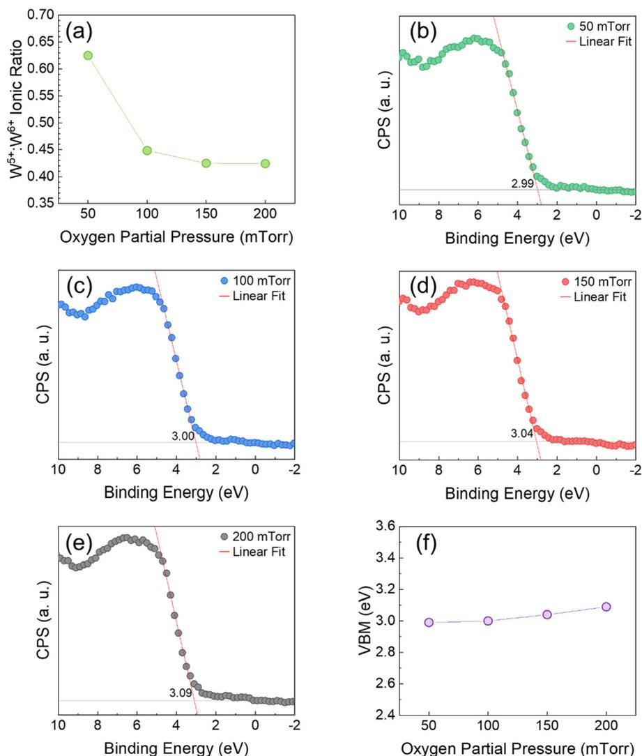
**Fig. 2** (a) Surface  $W^{5+}:W^{6+}$  ionic ratio of the W-incorporated  $\beta$ - $Ga_2O_3$  films as a function of  $pO_2$ . (b–e) Extrapolated valence band XPS spectra of the films and (f) variation in valence band maxima with increasing  $pO_2$ .
