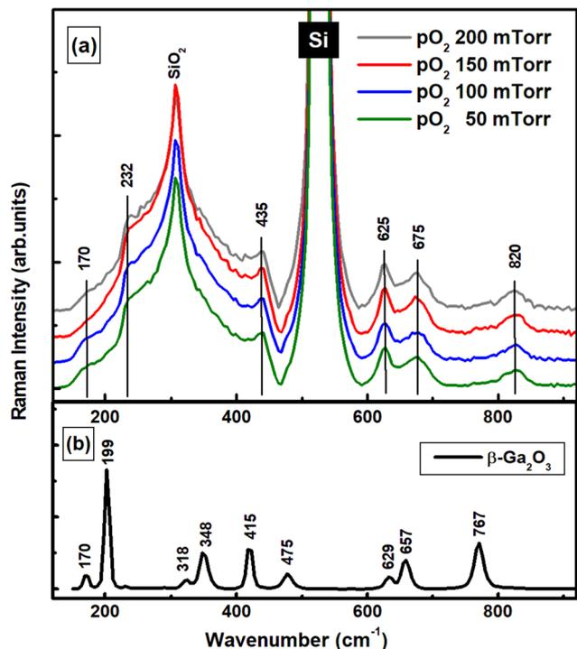
Fig. 3 (a) Raman spectra of W-incorporated  $\beta$ -Ga<sub>2</sub>O<sub>3</sub> films deposited under variable  $pO_2$ . (b) Raman spectrum of bulk  $\beta$ -Ga<sub>2</sub>O<sub>3</sub>.
