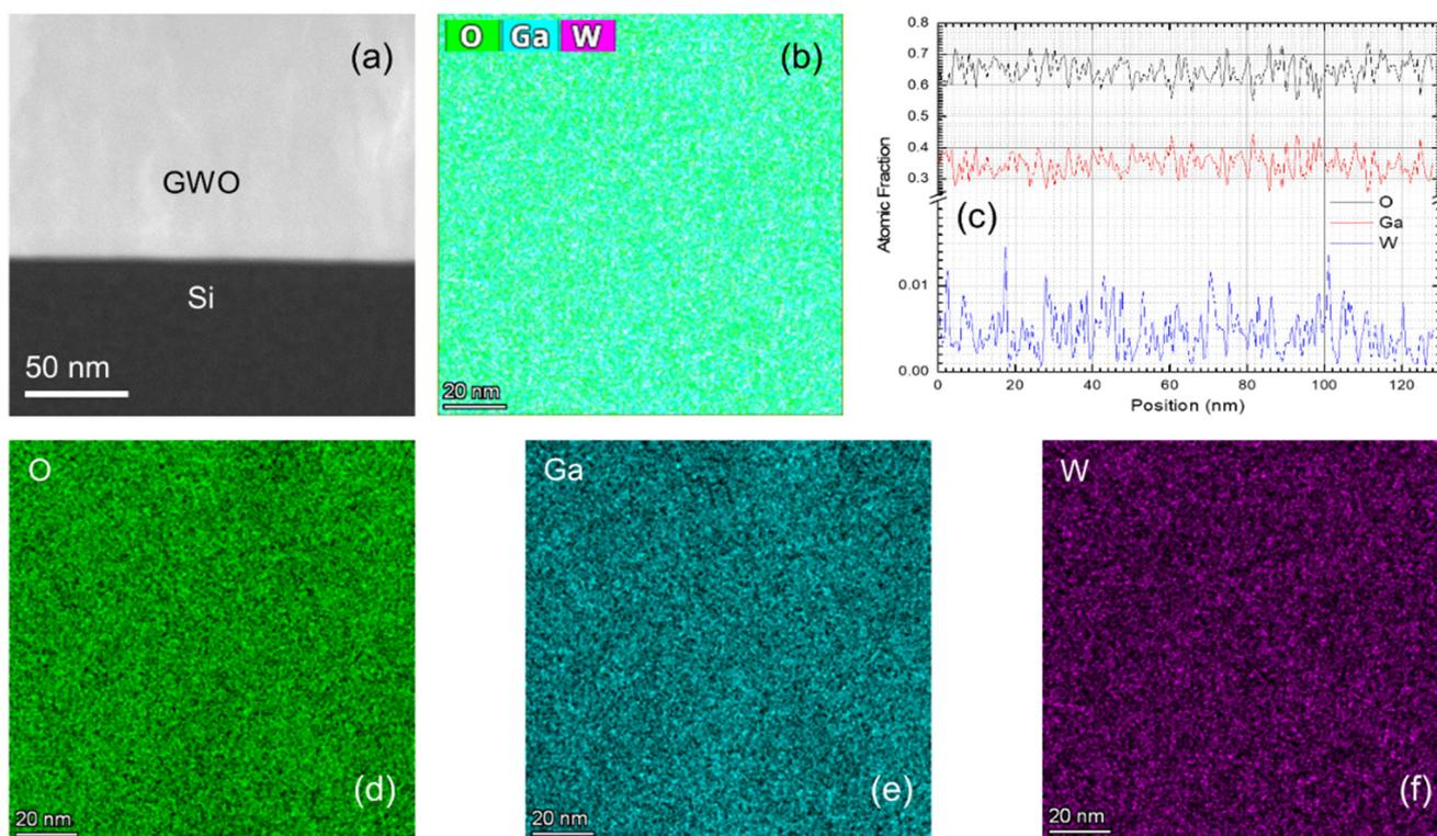
Fig. 5 Cross sectional TEM images: (a) high-resolution HAADF STEM images of W-incorporated  $\beta$ - $Ga_2O_3$  films on a Si platform. (b and c) Elemental color mapping and corresponding atomic fraction plots for Ga, O, and W, respectively. (d–f) Individual color mapping of O, Ga, and W.
