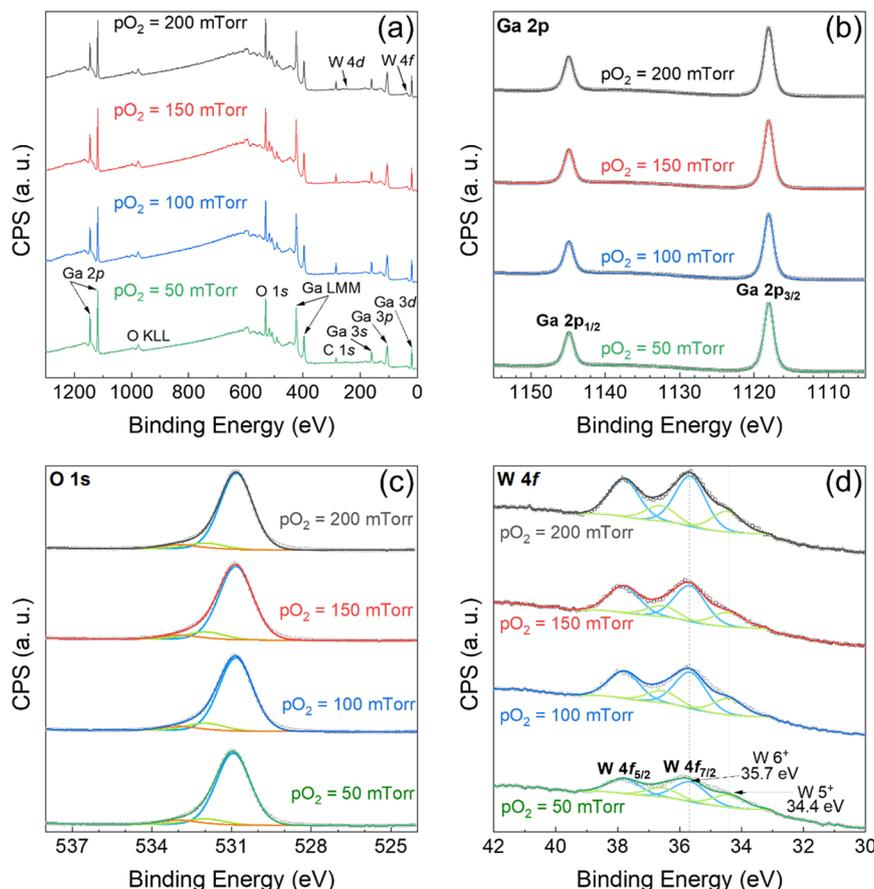
**Fig. 1** XPS data of the PLD W-incorporated  $\beta$ -Ga<sub>2</sub>O<sub>3</sub> films deposited at varying  $p$ O<sub>2</sub>. The data shown are: (a) survey XPS scan and high-resolution core level XPS spectra of (b) Ga 2p, (c) O 1s, and (d) W 4f. The data indicate a stable configuration of Ga ions irrespective of the  $p$ O<sub>2</sub> during deposition. The complex chemistry of W-ions depending on the  $p$ O<sub>2</sub> is evident from the data and analyses.
