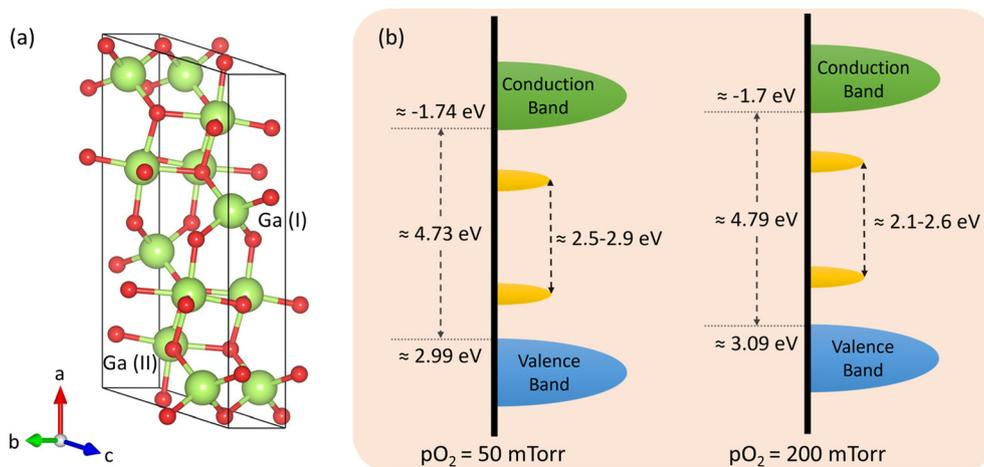
**Fig. 9** (a) Crystal structure of the monoclinic  $\beta$ - $\text{Ga}_2\text{O}_3$ . The inequivalent Ga(I) and Ga(II) sites refer to the tetrahedral and octahedral positions, respectively. (b) The schematic density of states diagram, calculated from XPS, UV-vis, and PL spectroscopy, of the W-incorporated  $\beta$ - $\text{Ga}_2\text{O}_3$  films grown under  $\text{O}_2$ -poor and  $\text{O}_2$ -rich conditions.
