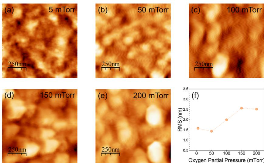
Fig. 4 AFM data of PLD GWO films deposited at varying  $pO_2$ . (a–e) AFM surface morphology scans; and (f) RMS roughness variation with  $pO_2$  for PLD GWO films. The effect of  $pO_2$  on the morphology and roughness of PLD GWO films is evident.
