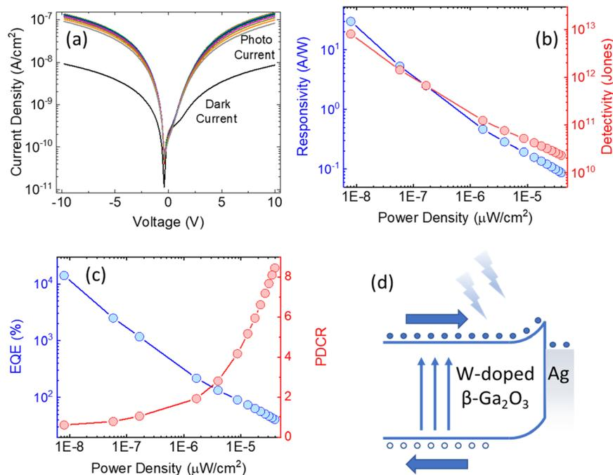
**Fig. 10** Steady-state response: (a) dark and photocurrent under forward/reverse bias; (b) incident power-dependent responsivity and detectivity at 265 nm irradiation and 10 V forward bias; (c) incident power-dependent EQE and PDCR at 265 nm irradiation and 10 V forward bias; (d) empirical band diagram at the interface of the metal-semiconductor junction.
