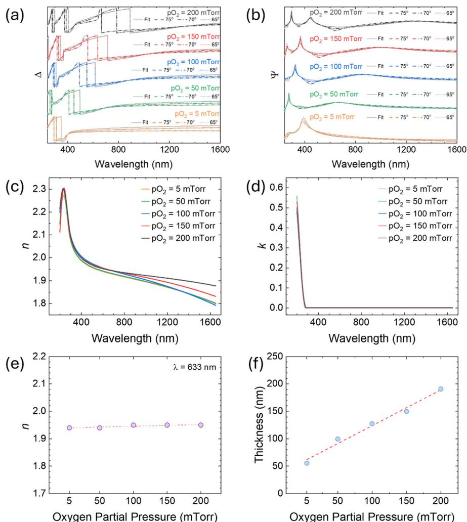
**Fig. 6** SE data of as-grown samples. (a and b) Representative plots of psi and delta functions extracted at different angles of incidence of the sample grown at varying  $p\text{O}_2$ . (c and d) Refractive index and extinction coefficient of all the samples. (e and f) Refractive index at a wavelength of 633 nm and pressure-dependent thickness variation of all the samples.
