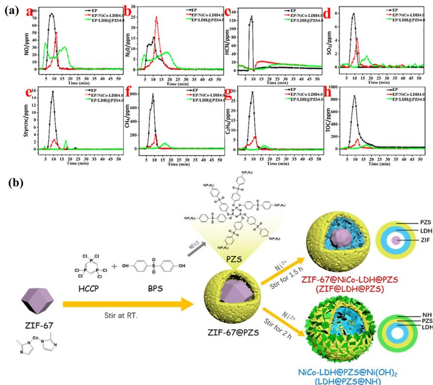
**Fig. 4** (a) Time curves showing the generation of harmful gases during combustion (a–h) for pure EP, EP/NiCo-LDH 4.0, and EP/NiCo-LDH@PZS 4.0. Reproduced from ref. 67 with permission from [American Chemical Society], copyright [2019]; (b) diagrammatic representation of the synthetic pathways for two samples with distinct nanostructures. Reproduced from ref. 69 with permission from [American Chemical Society], copyright [2022].
