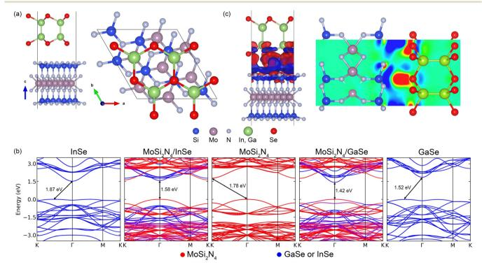
Fig. 1 (a) Atomic structure of MoSi<sub>2</sub>N<sub>4</sub>/MSe (M = Ga, In). (b) Band structures of the individual monolayers and the VDWH. (c) Charge transfer between the monolayers in the VDWHs. The blue region shows electron depletion, and the red region shows electron accumulation. Hence electrons transfer from MoSi<sub>2</sub>N<sub>4</sub> to GaSe (InSe).
