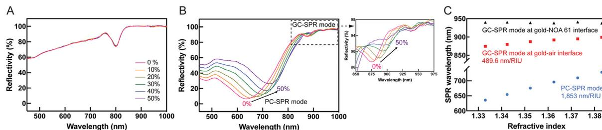
**Fig. 5** SPR reflectivity curves of an ethylene glycol aqueous solution (0–50% w/w,  $n = 1.33300$ – $1.38313$ ) were observed at incident angles of (A)  $45^\circ$  and (B)  $85^\circ$ . (C) Plots illustrating the excitation wavelength for SPR in PC-SPR mode (blue circle), GC-SPR mode at the gold–air interface (red square), and GC-SPR mode at the gold–NOA61 interface (black triangle) as a function of the refractive index.
