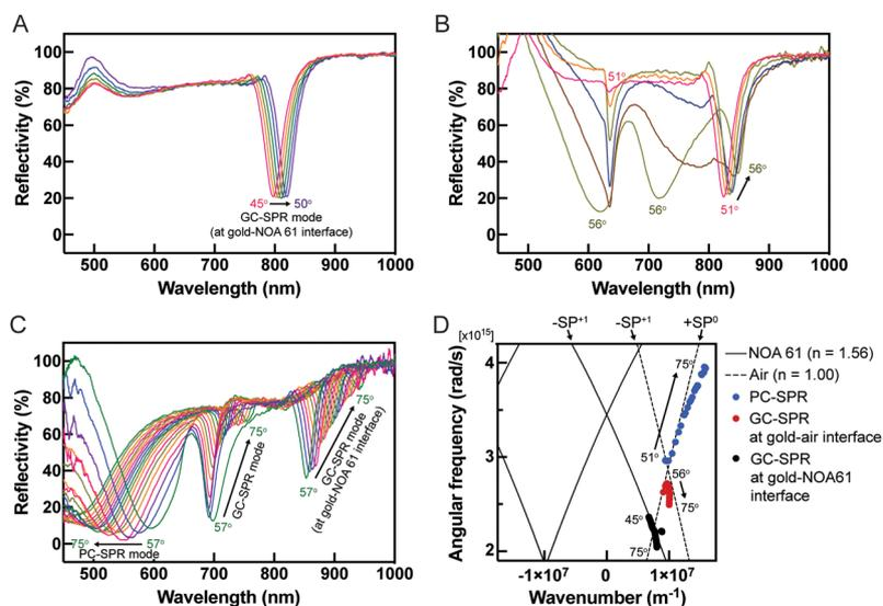
**Fig. 3** SPR reflectivity curves in the air ( $n = 1.000028$ ) of the dual-mode SPR sensor chip at various incident angles: (A) 45–50°, (B) 51–56°, and (C) 57–75°. (D) Experimental results of dual-mode SPR, encompassing PC-SPR mode (blue dots), GC-SPR mode at the gold–air interface (black dots), and GC-SPR mode at the gold–NOA 61 interface (red dots), and calculated results of the dispersion of SPs at the gold–NOA 61 (full lines) and gold–air (dash line) interfaces.
