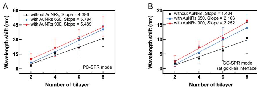
Fig. 9 Comparison of linear regression plots depicting the relationship between the number of PDADMAC/PSS bilayers and the wavelength shift in both (A) the PC-SPR mode and (B) the GC-SPR mode at the gold-air interface. Three distinct scenarios are represented in the plots: no AuNRs added (black dots), AuNRs 650 added (blue dots), and AuNRs 900 added (red dots).
