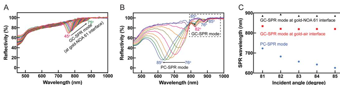
Fig. 4 SPR reflectivity curves in an aqueous solution ( $n = 1.33300$ ) of the dual-mode SPR sensor chip at various incident angles: (A)  $45\text{--}75^\circ$  and (B)  $76\text{--}85^\circ$ . (C) Plots illustrating the SPR wavelength excitation of PC-SPR (blue circle), GC-SPR mode at the gold–air interface (red square), and GC-SPR mode at the gold–NOA61 interface (black triangle) as a function of the incident angle within the range of  $81\text{--}85^\circ$ .
