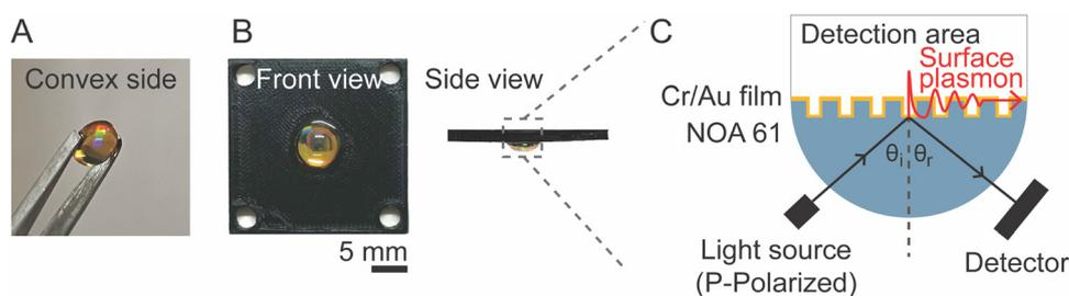
**Fig. 1** (A) Grating diffraction pattern on convex side of NOA 61 polymeric grating prism (B) front and side views of the dual-mode SPR sensor chip. (C) Schematic representation of the internal microfluidic cell structure, illustrating the underlying mechanisms governing the SPR excitation process within the dual-mode SPR sensor chip.
