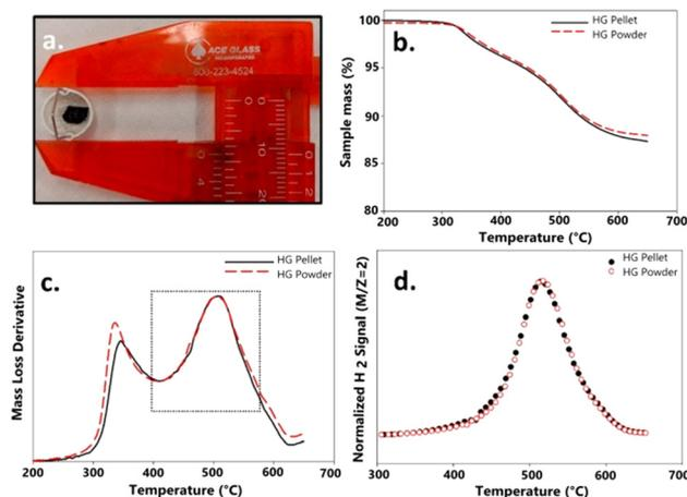
**Fig. 7** (a) Photograph of compressed hydrogenated graphite (HG) in a TGA pan. (b) TGA for HG pellets and HG powder. (c) Differential thermogravimetric analysis (DTG) for HG pellet and powder. (d) TGA-MS profile for  $m/z$  of 2 of HG pellets and powder samples. This figure has been reproduced from ref. 194 with permission from Elsevier, copyright 2021.
