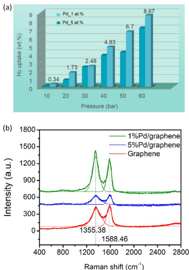
**Fig. 8** (a) Hydrogen uptake capacities of 1% Pd/graphene and 5% Pd/graphene functionalized graphene at various charging pressures. (b) Raman spectroscopy of graphene, 1% Pd/graphene, and 5% Pd/graphene, showing D and G bands at  $\sim 1355.38$   $\text{cm}^{-1}$  and  $\sim 1588.46$   $\text{cm}^{-1}$ , respectively. This figure has been reproduced from ref. 106 with permission from American Chemical Society, copyright 2016.
