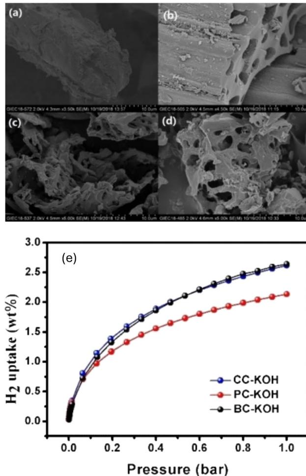
Fig. 14 SEM image of carbon derived from cornstalk (CC), after (a) thermal activation at 800 °C, (b) ZnCl<sub>2</sub> activation, (c) H<sub>3</sub>PO<sub>4</sub> activation and (d) KOH activation. (e) H<sub>2</sub> adsorption for the KOH activated carbons derived from bagasse, cornstalk and pine powder shown. This figure has been reproduced from ref. 133 with permission from John Wiley and Sons, copyright 2020.
