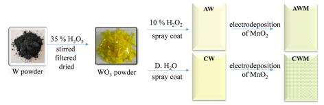
Fig. 1 Schematic representation of the fabrication process of MnO<sub>2</sub> coated WO<sub>3</sub> thin film electrodes.
