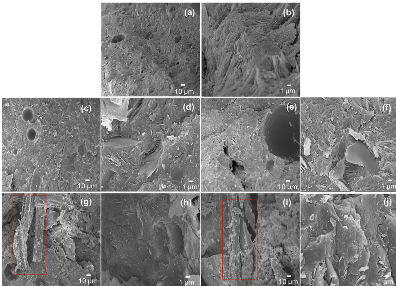
**Fig. 3** SEM pictures of geopolymer and geopolymer-sawdust composites at two magnifications ( $\times 500$  and  $\times 5000$ ). (a) and (b) G, (c) and (d) G-TS2, (e) and (f) G-S2, (g) and (h) G-TS10 and (i) and (j) G-S10.
