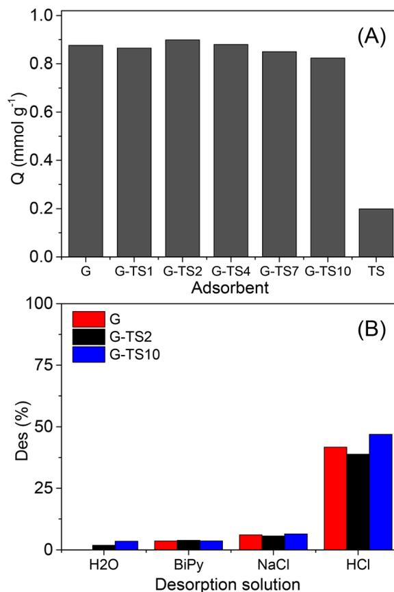
Fig. 8 (A) Variation of Co(II) adsorption capacity of treated sawdust (TS), geopolymer and geopolymer-sawdust (treated and untreated) composites with particle sizes 400–250  $\mu\text{m}$ . Experimental conditions: 0.2 g of adsorbent in 100 mL of Co(II) 3 mM, stirred for two days at 250 rpm. (B) Co(II) desorption percentages as a function of desorption solution. Experimental conditions: 2.5 mg of loaded adsorbent in 5 mL of desorbing solution, stirred at 250 rpm for 1 day.
