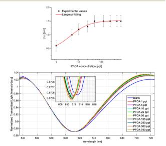
Fig. 6 Test results by Pitruzzella et al. for their MIP sensor within a simulated seawater matrix. The data readings (top) combined with the change in the observed wavelength with increasing concentration (bottom) indicate that the sensitivity of the sensor decreases with higher concentrations.
