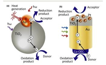
Fig. 7 Examples of non-sensor based plasmonic technologies. (a) Plasmonic gold (Au) nanoparticle acts as an electron sink for excited semiconductor electrons as well as an independent electron generator for a more efficient photoactive catalyst. (b) A collection of gold nanoparticles excited *via* light generates SPR electrons which are then used within the electrochemical cell.<sup>35</sup>
