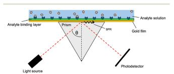
Fig. 2 Depiction of the SPR sensor technology in a Kretschmann configuration. A specific angle of reflectance will instigate SPR, causing a decrease in measured light intensity. As the analyte binds, the angle at which SPR occurs will shift. This figure was created by the authors.
