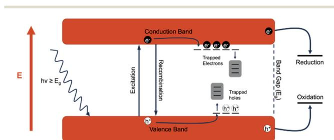
**Fig. 8** Diagram depicting the absorbance of a photon in a semiconducting material, resulting in the generation of an exciton. The generated electron exists within the conduction band, whereas the hole exists within the valence band. By 'trapping' either the conduction band electron or valence hole, the lifetime of the generated exciton pair can be elongated. Generated electrons undergo reduction and generated holes undergo oxidation. This figure was created by the authors.
