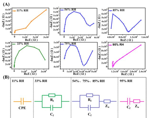
Fig. 10 (A) Complex impedances and (B) corresponding equivalent circuit models of the ZG-Ag-2 sensor.
