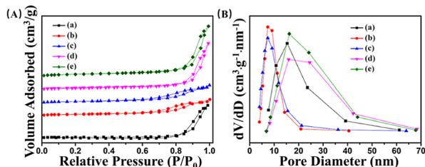
**Fig. 6** (A)  $\text{N}_2$  adsorption-desorption isotherms and (B) pore size distributions of (a) ZG, (b) ZG-Ag-1, (c) ZG-Ag-2, (d) ZG-Ag-3 and (e) ZG-Ag-4.
