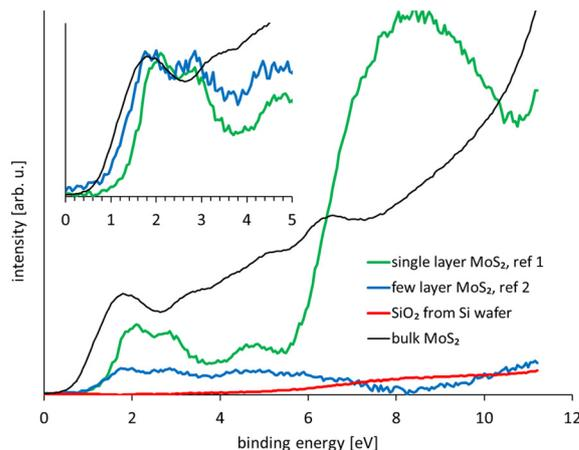
Fig. 6 Spectra of the components forming the  $\text{MoS}_2/\text{Si}/\text{SiO}_2$  sample: the monolayer  $\text{MoS}_2$ , few layer  $\text{MoS}_2$  and the  $\text{Si}/\text{SiO}_2$  substrate. For reference a spectrum of bulk  $\text{MoS}_2$  is shown. In the inset the onset of the VB are shown. In the inset spectra are scaled such that they have the same intensity at their first maximum around 1 to 1.5 eV.
