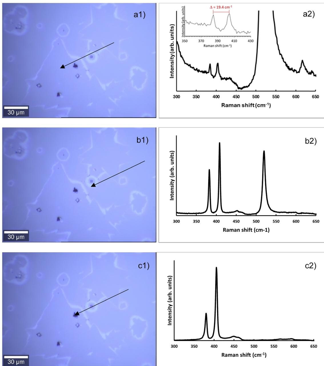
Fig. 2 Optical images (a1–c1) and Raman spectra (a2–c2) of specific areas on the optical image. In a1 an inset with the  $E_{2g}^1$  and  $A_{1g}$  modes are shown. In a2 an inset is shown with the separation of the  $E_{2g}^1$  and  $A_{1g}$  modes.
