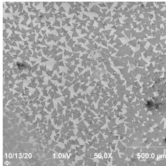
**Fig. 1** SEM image of the central area of the sample shown in Fig. S1†. The dark grey triangular shaped areas are the monolayer MoS<sub>2</sub> crystallites. The crystallites show a small degree of overlap. The relative fraction of the sample surface formed by the substrate, monolayer and few layer MoS<sub>2</sub> is provided in Table 1.
