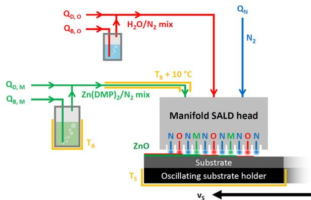
**Fig. 2** Schematic of the close-proximity SALD setup at LMGP. At the substrate surface, three types of gas regions exist corresponding to the metal precursor in green (M), the oxygen source in red (O), and the inert nitrogen gas barrier (N). Heaters are schematically colored in gold.
