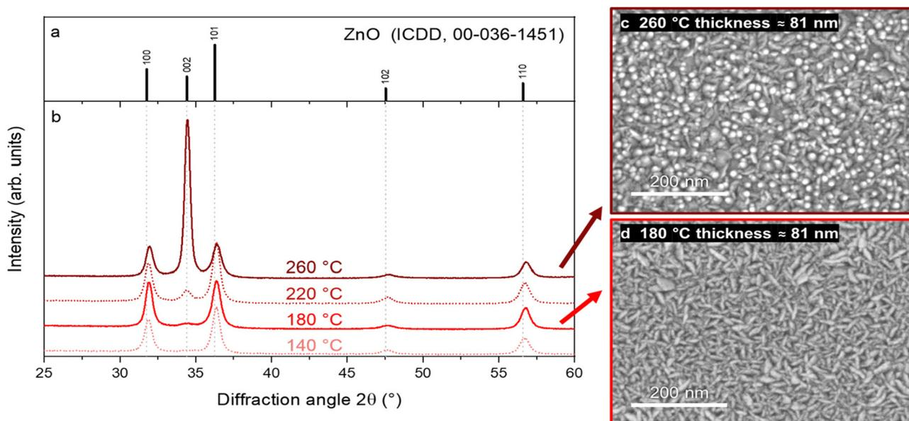
**Fig. 4** GIXRD patterns of ZnO thin films deposited at various temperatures (b) compared with the theoretical diffraction pattern for ZnO in the wurtzite structure as per the ICDD database (a). The thin films showed mainly *a*-axis growth for all temperatures except 260 °C where *c*-axis growth was achieved. This texture change is visible in the surface morphology as studied using SEM on samples grown at 260 °C (c) and 180 °C (d).
