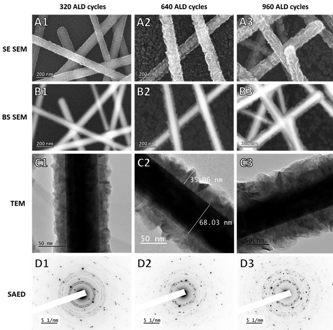
**Fig. 6** Evolution of ZnO coating morphology after 320 (–1), 640 (–2), and 960 (–3) ALD cycles at 150 °C using Zn(DMP)<sub>2</sub>, studied using SE SEM for surface morphology (A1–A3), BS SEM for chemical contrast inside nanowire (B1–B3), TEM of single nanowires to show morphological detail (C1–C3), and SAED to show ZnO coating crystallinity (D1–D3).
