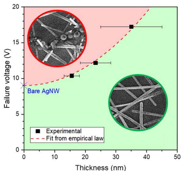
Fig. 7 Evolution of failure voltage vs. ZnO coating thickness around AgNWs, with the green region corresponding to a percolating network and the red region to non-percolating networks (*i.e.* after failure), and fitting our data with eqn (1).
