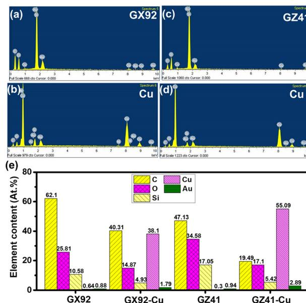
**Fig. 5** Elemental distribution pattern on the surface of ABF and copper layer after peeling: (a) GX film; (b) copper plated GX film; (c) GZ film; (d) copper plated GZ film; (e) comparison of element contents.
