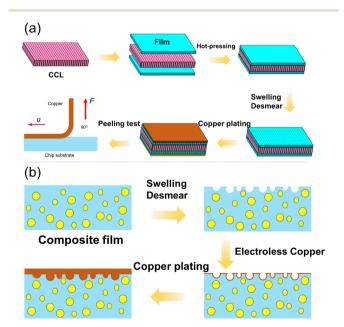
Fig. 1 Schematic diagram of (a) the whole fabrication process of chip substrates and (b) preparation processes of copper/epoxy composite films.
