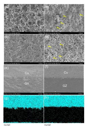
Fig. 4 The surface SEM images of the film and copper after peeling: (a) GX film and (b) planted copper; (c) GZ film and (d) plated copper. Cross section SEM images of (e) GX and (f) GZ samples; EDS elemental mappings of (g) GX and (h) GZ samples.
