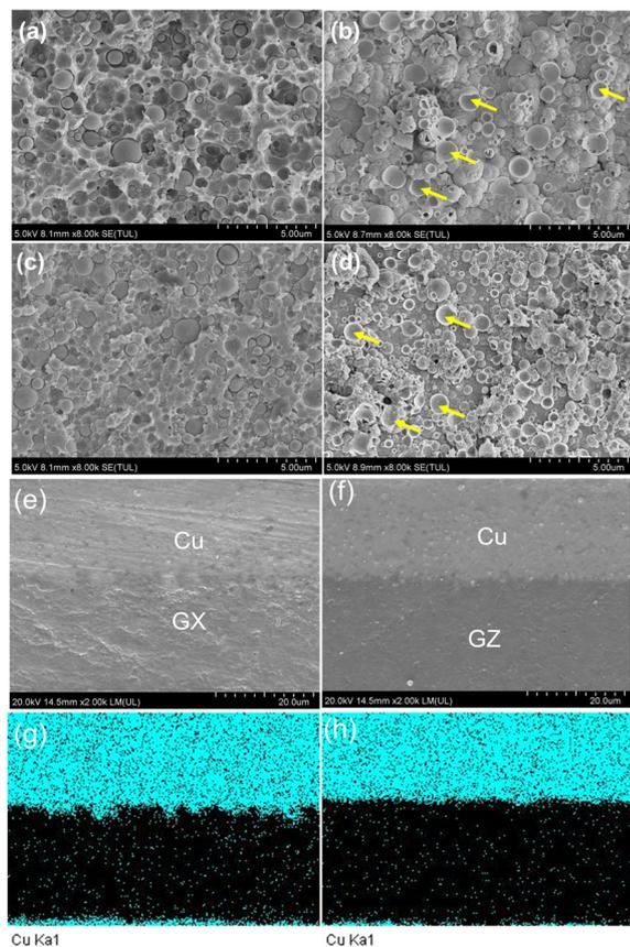
**Fig. 4** The surface SEM images of the film and copper after peeling: (a) GX film and (b) planted copper; (c) GZ film and (d) plated copper. Cross section SEM images of (e) GX and (f) GZ samples; EDS elemental mappings of (g) GX and (h) GZ samples.
