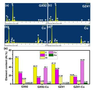
Fig. 5 Flemental distribution pattern on the surface of ABF and copper layer after peeling: (a) GX film; (b) copper plated GX film; (c) GZ film; (d) copper plated GZ film; (e) comparison of element contents.
