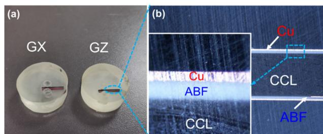
Fig. 2 (a) Samples sealed in epoxy resin; (b) the microstructure of chip substrates.
