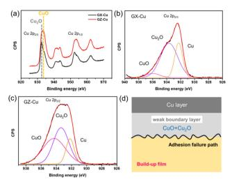
Fig. 6 Cu 2p XPS spectra and adhesion failure mechanism: (a) Cu 2p peak of peeled copper strips; (b) Cu 2p<sub>3/2</sub> of the GX film; (c) Cu 2p<sub>3/2</sub> of the GZ film; (d) schematic diagram of the adhesive failure interface between copper and the polymer composite
