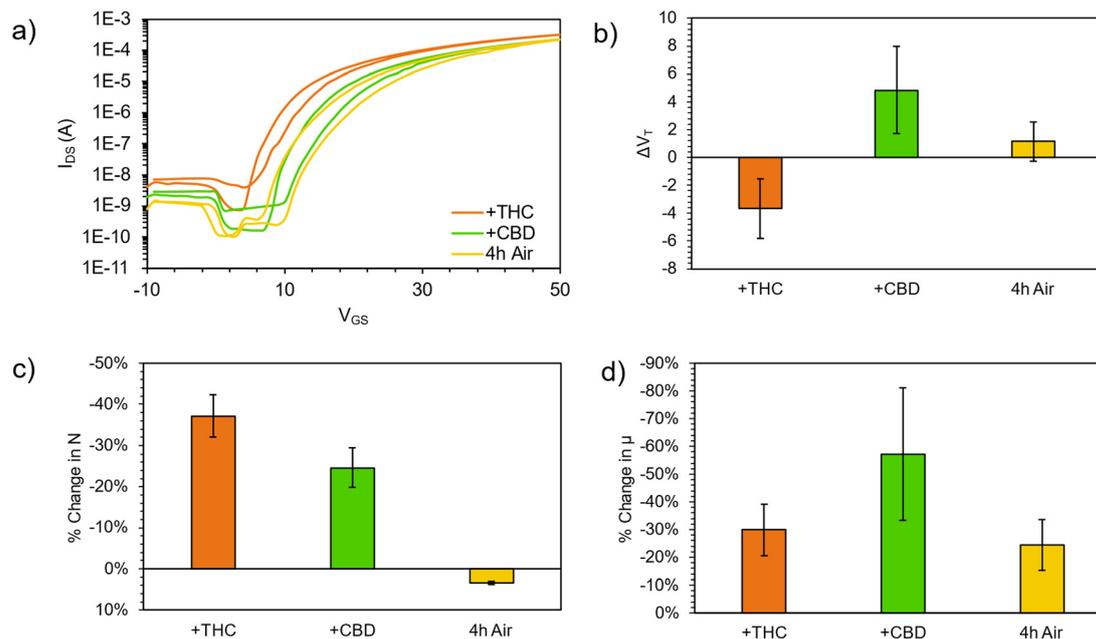
**Fig. 2**  $(F_5PhO)_2-F_{16}-SiPc$  performance after exposure to THC and CBD, or after 4 h of air exposure as a control, demonstrated by the (a) transfer curve ( $V_{SD} = 50$  V) of a representative device, (b) average change in threshold voltage,  $V_T$ , (c) average change in defect density,  $N$ , and (d) the average change in electron mobility,  $\mu_e$ . All averages are for a minimum of 10 transistors.
