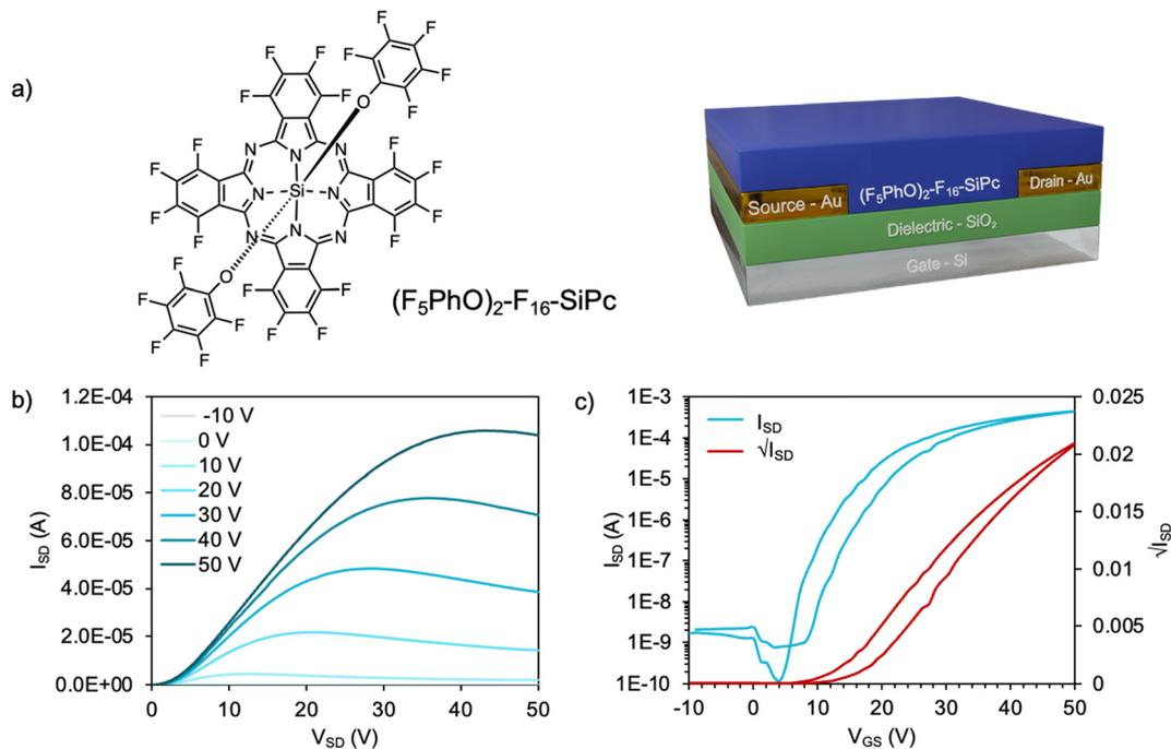
Fig. 1 (a) (F<sub>5</sub>PhO)<sub>2</sub>-F<sub>16</sub>-SiPc chemical structure, and the bottom-gate bottom-contact (BGBC) device architecture used in this study, along with the associated (b) output curves and (c) transfer curves ( $V_{SD} = 50$  V) of the (F<sub>5</sub>PhO)<sub>2</sub>-F<sub>16</sub>-SiPc OTFTs tested in air.
