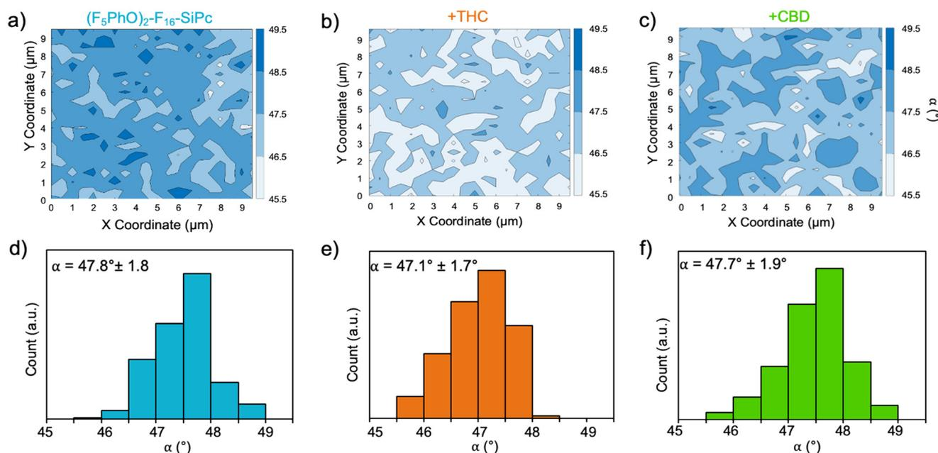
Fig. 4 Polarized Raman microscopy mapping on a  $10 \times 10 \mu m$  area with a  $0.5 \mu m$  step size to generate a contour plot of the average  $(F_5PhO)_2-F_{16}-SiPc$  angle to the surface, with the angle distribution for the (a and d) baseline  $(F_5PhO)_2-F_{16}-SiPc$  film, (b and e) after exposure to THC, and (c and f) after exposure to CBD.
