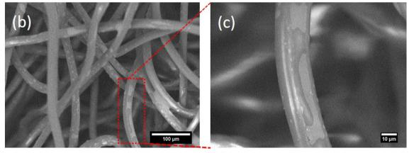
Fig. 6 SEM images of (a) uncoated PP felt, (b) PP felt coated with PEI at 1.0 μmol N per cm² (×250) and (c) PP felt coated with PEI at 1.0 μmol N per cm2 (×1000).
