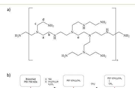
Fig. 1 (a) Chemical structure of branched PEI (750 kDa); (b) schematic route to alkylated PEIs synthesis
