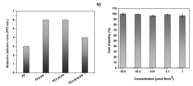
Fig. 7 a) Reduced viral titer of FCV after 4 hours incubation with uncoated PP and PP felt coated with PEI, PEI-H, and PEI-HM at a concentration of  $1 \times 10^{-4}$  µmol N per cm<sup>2</sup> (the error bar is too small to display), and b) cell viability of CFRK cells after 4 hours of incubation with PP felt coated with PEI-HM at different concentrations (tests were conducted in triplicate).
