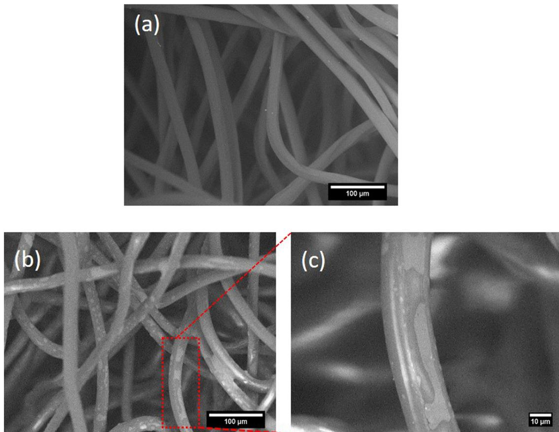
Fig. 6 SEM images of (a) uncoated PP felt, (b) PP felt coated with PEI at  $1.0 \mu\text{mol N per cm}^2$  ( $\times 250$ ) and (c) PP felt coated with PEI at  $1.0 \mu\text{mol N per cm}^2$  ( $\times 1000$ ).
