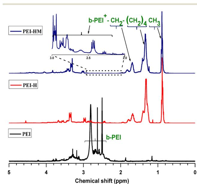
Fig. 3 <sup>1</sup>H-NMR spectra of the prepared PEI and alkylated PEI derivatives.
