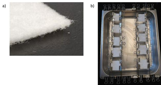
Fig. 2 (a) Image of PP fiber filtration felt and (b) assembly for the deposition of PEI and alkylated PEI derivatives at a concentration of  $1 \times 10^{-4}$   $\mu\text{mol N}$  per  $\text{cm}^2$ .
