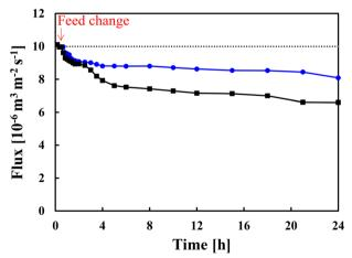
Fig. 5 Time-course of the flux when pre-treated real seawater was fed through unmodified (black, squares) and grafted (blue, circles) membranes with a grafting amount of 0.12 mg cm<sup>-2</sup>. The dotted line indicates an ideal flux through an unfouled membrane.
