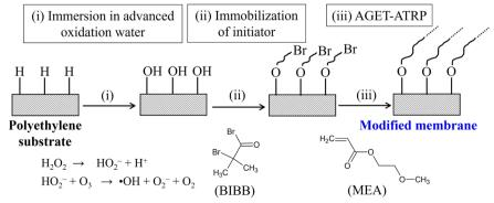
Fig. 1 Schematic illustration of the modification
