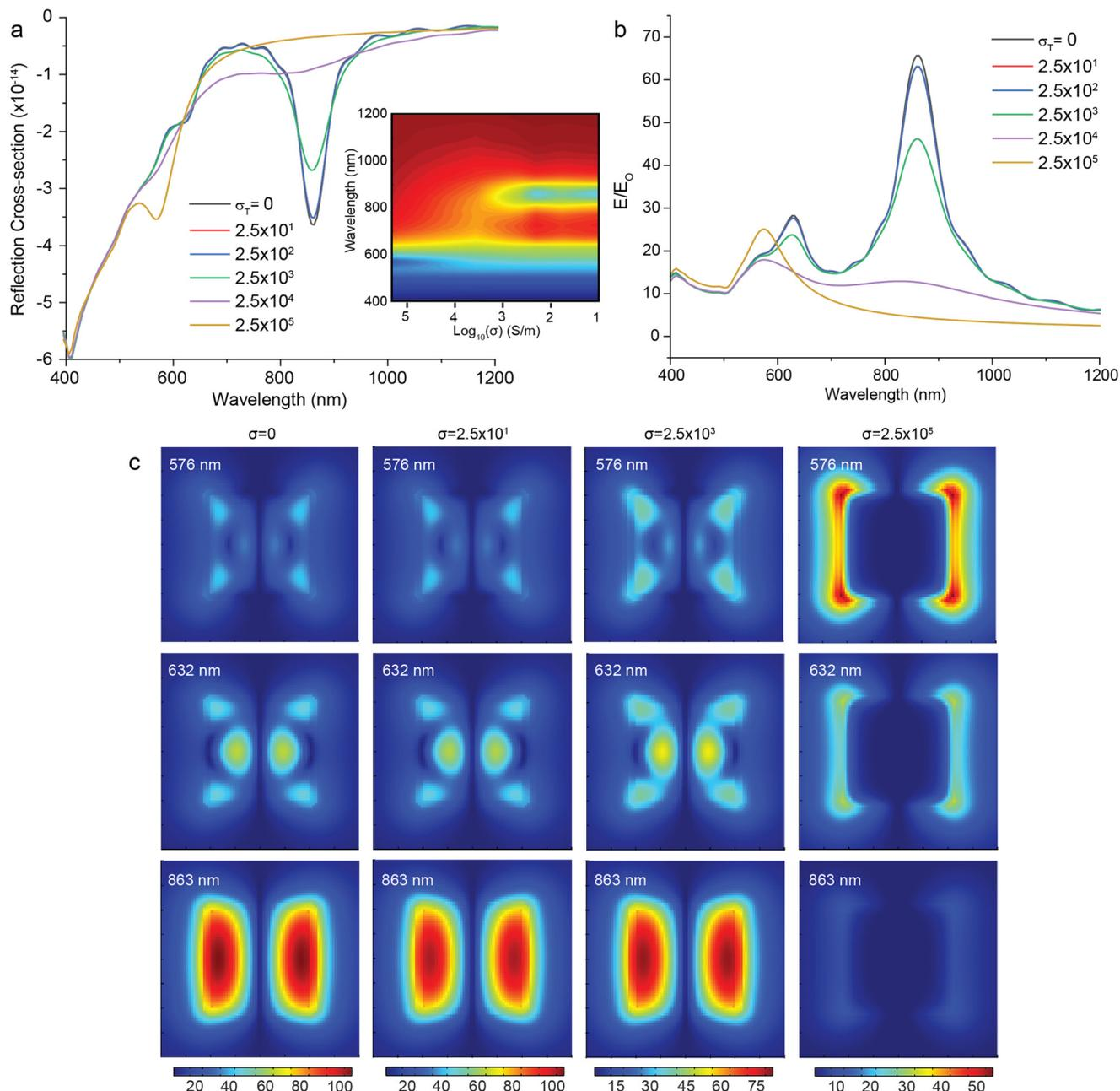
**Fig. 2** Simulated quantum correction model metasurface: (a) simulated reflectance spectra for metasurface with constant gap height (2 nm) and varied conductivity  $\sigma_T$ , insert is reflectance intensity map for metasurface with different conductivity (b) simulated average electric field enhancements for metasurface with constant gap height (2 nm) and varied conductivity  $\sigma_T$ . (c) Near-field distribution for metasurface with different conductivity  $\sigma_T$ .
