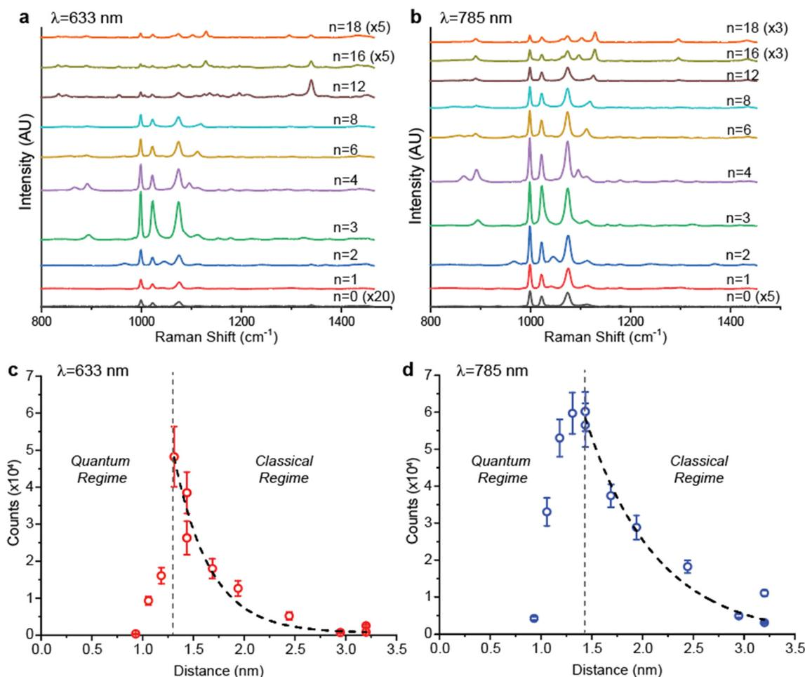
**Fig. 4** SERS measurement and distance dependent Raman intensity: (a) Raman spectra for metasurface separated by different chain length alkanethiol at 633 nm excitation. (b) Raman spectra for metasurface separated by different chain length alkanethiol at 785 nm excitation. (c) Gap distance dependent Raman intensity at 633 nm excitation. (d) Gap distance dependent Raman intensity at 785 nm excitation.
