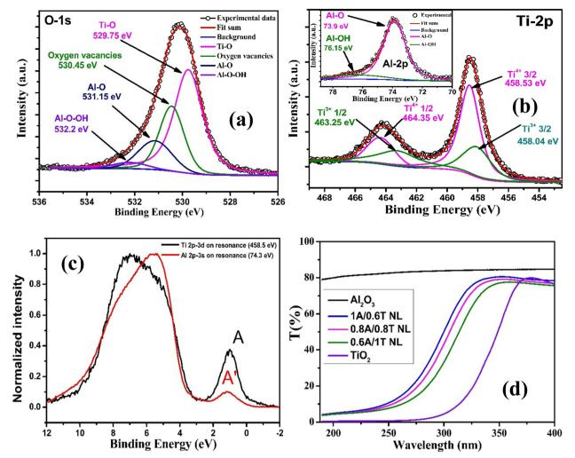
Fig. 4 The measured and deconvoluted (a) O 1s, (b) Ti 2p, (inset) Al 2p core levels XPS spectra of 0.8A-0.8T NL, (c) the recorded Al 2p-3s and Ti 2p-3d VB-RPES spectra of 0.8A-0.8T NL at the resonance photon excitation energy of ~458.5 eV and 74.3 eV respectively. (d) Transmission vs. wavelength spectra of ~60 nm TiO<sub>2</sub>, Al<sub>2</sub>O<sub>3</sub> film and for three ~60 nm thick representative NLs, i.e. 1A/0.6T, 0.8A/0.8T and 0.6A/1T NL
