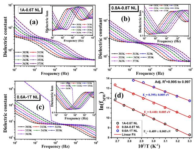
Fig. 3 Frequency dispersed  $\varepsilon_r$  and  $\tan \delta$  spectra for (a) 1A-0.6T NL, (b) 0.8A-0.8T NL and (c) 0.6A-1T NL measured in a temperature range from 303 K to 373 K are depicted in the main figure and inset, respectively. (d) Arrhenius linear curve fitting for M-W relaxation peak position variation with experimental temperature with adj. R<sup>2</sup> values close to unity.
