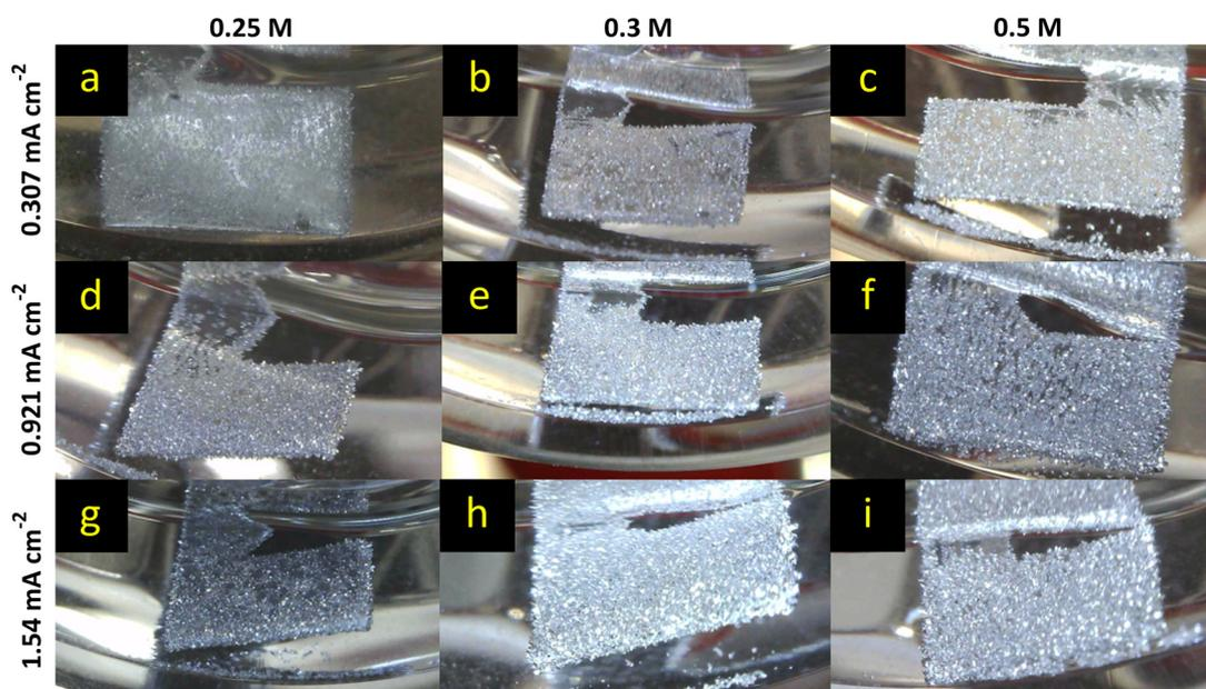
**Fig. 2** Mg deposition using the benchmark Grignard electrolyte MeMgCl in THF as a function of current density (rows) and concentration (columns) after 8 h of chronopotentiometry. The applied current density ranged from  $0.307 \text{ mA cm}^{-2}$  (a–c) to  $0.921 \text{ mA cm}^{-2}$  (d–f) and  $1.54 \text{ mA cm}^{-2}$  (g–i) for MeMgCl concentrations between 0.25 M and 0.5 M.
