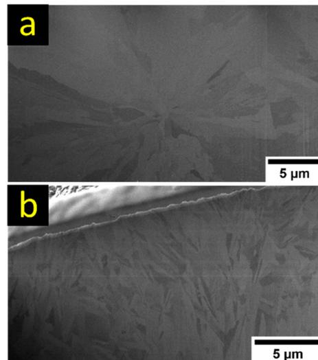
**Fig. 12** Ion-induced SEM images of FIB cross sections of Mg deposits from 0.2 M Mg(HMDS)<sub>2</sub>-2AlCl<sub>3</sub> (a) and 0.2 M Mg[B(hfip)<sub>4</sub>]<sub>2</sub> (b) electrolyte solutions obtained with a current density of 0.307 mA cm<sup>-2</sup>.
