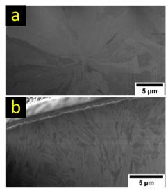
Fig. 12 Ion-induced SEM images of FIB cross sections of Mg deposits from 0.2 M Mg(HMDS)<sub>2</sub>-2AlCl<sub>3</sub> (a) and 0.2 M Mg[B(hfip)<sub>4</sub>]<sub>2</sub> (b) electrolyte solutions obtained with a current density of 0.307  $mA cm^{-2}$ .
