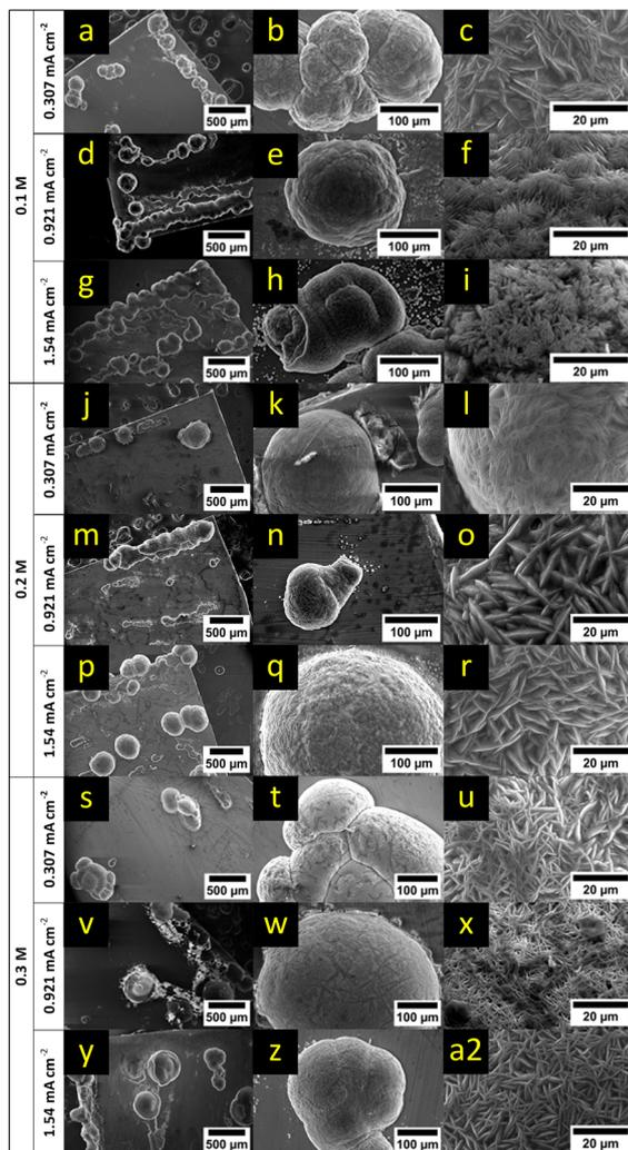
Fig. 7 SEM images after 8 h of magnesium deposition from a 0.1 M (a–i), 0.2 M (j–r) and 0.3 M (s–a2)  $\text{Mg}(\text{HMDS})_2\text{-}2\text{AlCl}_3$  electrolyte solution. The applied current density (rows) can be derived from the subsection of each concentration.
