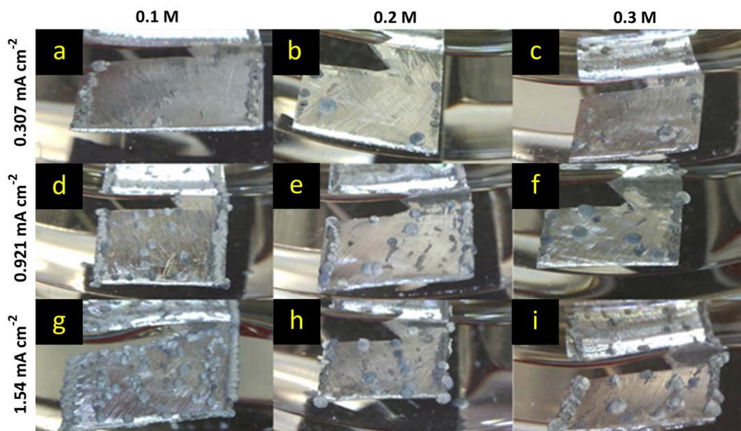
Fig. 6 Mg deposition using the Mg(HMDS)<sub>2</sub>-2AlCl<sub>3</sub> electrolyte in THF as a function of current density (rows) and concentration (columns) after 8 h of chronopotentiometry. The applied current density ranged from 0.307 mA cm<sup>-2</sup> (a-c) to 0.921 mA cm<sup>-2</sup> (d-f) and 1.54 mA cm<sup>-2</sup> (g-i) for electrolyte concentrations between 0.1 M and 0.3 M.
