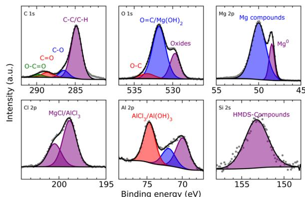
Fig. 8 C 1s (top left), O 1s (top middle), Mg 2p (top right) and Cl 2p (bottom left), Al 2p (bottom middle) and Si 2s (bottom right) XPS detail spectra of deposited Mg after 8 h from a 0.1 M  $\text{Mg}(\text{HMDS})_2\text{-}2\text{AlCl}_3$  solution with a current density of 1.54  $\text{mA cm}^{-2}$ .
