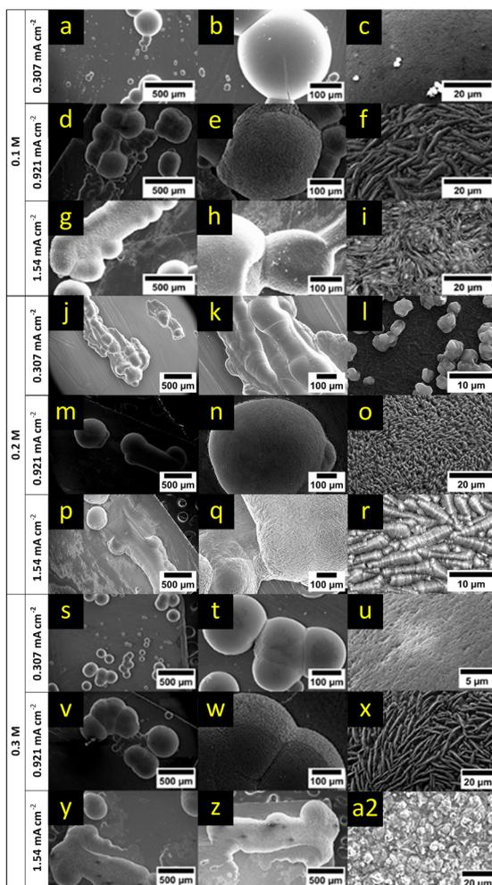
**Fig. 10** SEM images after 8 h of magnesium deposition from a 0.1 M (a–i), 0.2 M (j–r) and 0.3 M (s–a2)  $\text{Mg}[\text{B}(\text{hfp})_4]_2$  electrolyte solution. The applied current density (rows) can be derived from the subsection of each concentration.
