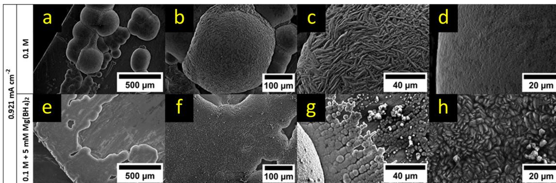
**Fig. 13** SEM comparison of magnesium deposits from a 0.1 M  $\text{Mg}[\text{B}(\text{hfip})_4]_2$  solution (a–d) and a  $\text{Mg}[\text{B}(\text{hfip})_4]_2$  solution containing 5 mM  $\text{Mg}(\text{BH}_4)_2$  (e–h). The pictures (a)–(c) were already presented in Fig. 10d–f but were reused for better comparability with the additive. Pictures (c and d) show the surface of the largest and one of the smaller deposits featured in (b), respectively.
