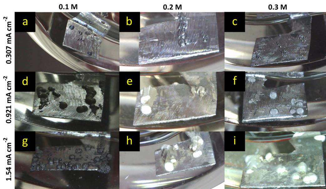
Fig. 9 Mg deposition using the  $\text{Mg}[\text{B}(\text{hfip})_4]_2$  electrolyte in DME as a function of current density (rows) and concentration (columns) after 8 h of chronopotentiometry. The applied current density ranged from 0.307  $\text{mA cm}^{-2}$  (a–c) to 0.921  $\text{mA cm}^{-2}$  (d–f) and 1.54  $\text{mA cm}^{-2}$  (g–i) for electrolyte concentrations between 0.1 M and 0.3 M.
