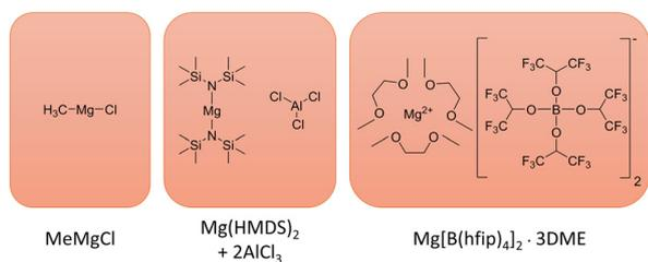
**Fig. 1** Structures of the  $\text{MeMgCl}$ ,  $\text{Mg}(\text{HMDS})_2$ – $2\text{AlCl}_3$  and  $\text{Mg}[\text{B}(\text{hfip})_4]_2$ – $3\text{DME}$  electrolytes. In the case of  $\text{Mg}(\text{HMDS})_2$ – $2\text{AlCl}_3$  electrolyte, only the precursors are drawn, as a complex Schlenk equilibrium unfolds upon dissolving in a respective solvent. A detailed investigation of this behaviour was performed by Merrill and Schaefer.<sup>18</sup>
