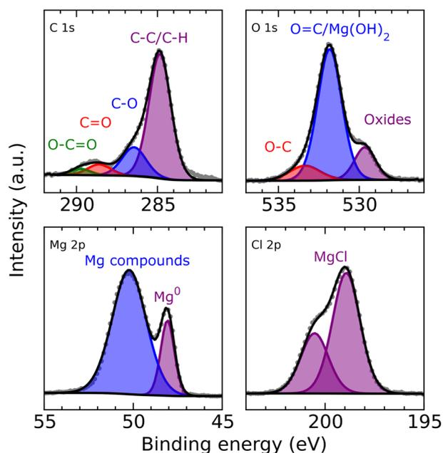
Fig. 5 C 1s (top left), O 1s (top right), Mg 2p (bottom left) and Cl 2p (bottom right) XPS detail spectra of deposited Mg after 8 h from a 0.25 M MeMgCl–THF solution with a current density of 1.54 mA cm<sup>-2</sup>.
