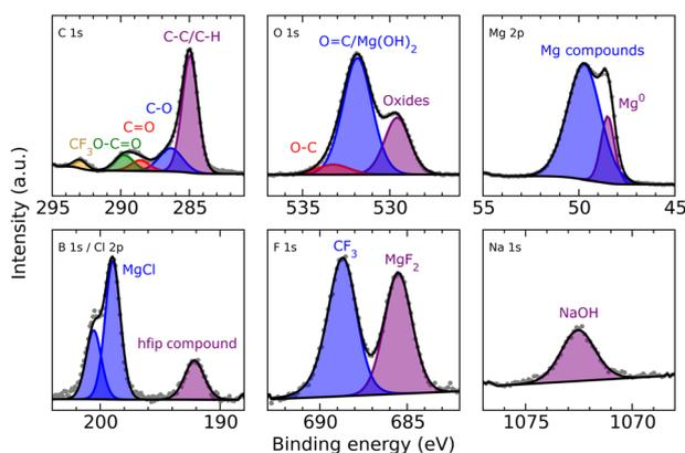
**Fig. 11** C 1s (top left), O 1s (top middle), Mg 2p (top right) and B 1s (bottom left), F 1s (bottom middle) and Na 1s (bottom right) XPS of deposited Mg after 8 h from a 0.1 M Mg[B(hfip)<sub>4</sub>]<sub>2</sub>-DME solution with a current density of 1.54 mA cm<sup>-2</sup>.
