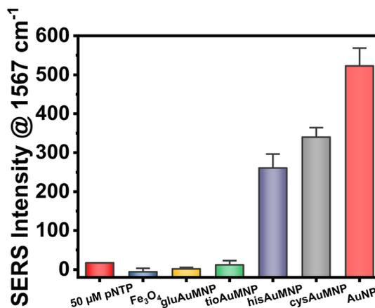
**Fig. 7** A bar chart depicting the Raman/SERS intensity from the 50 μM *p*-NTP on its own or when added to a solution of nanoparticle. The adsorption of *p*-NTP to the cysAuMNP, hisAuMNP, and AuNP were the only cases in which positive SERS enhancement was demonstrated, with AuNP having the highest increase overall. All measurements were completed in triplicate.
