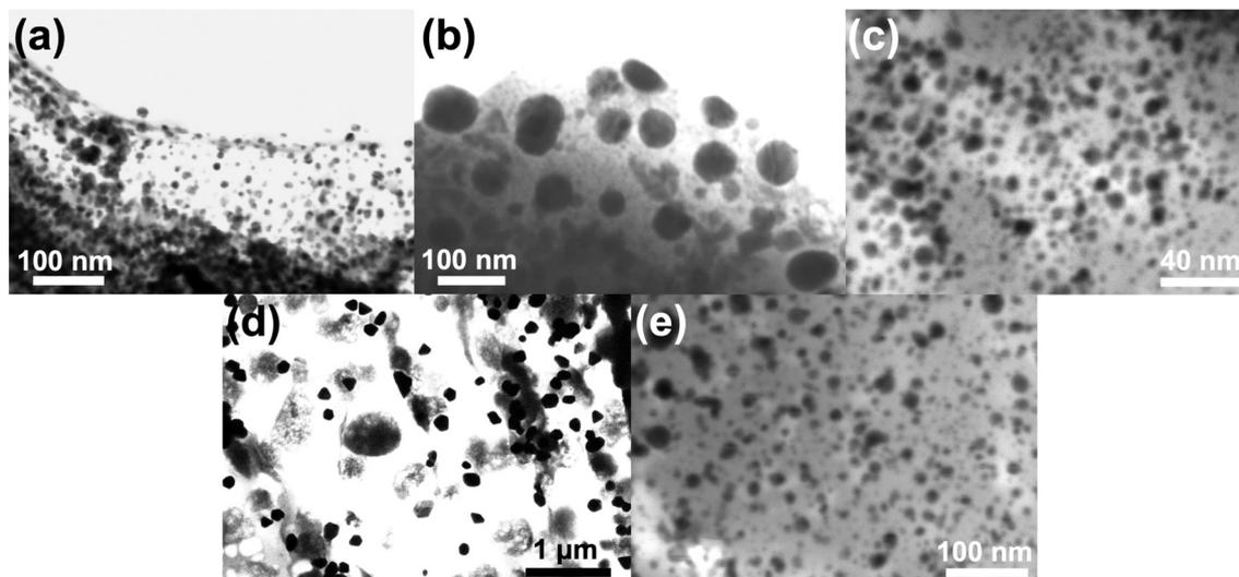
Fig. 5 STEM images of all nanoparticles synthesized. (a) Bare  $\text{Fe}_3\text{O}_4$ , (b) cysAuMNP, (c) gluAuMNP, (d) hisAuMNP, and (e) tioAuMNP. All images were obtained in bright-field mode on a STEM3+ detector at 30 kV accelerating voltage and 13–50 pA of current.
