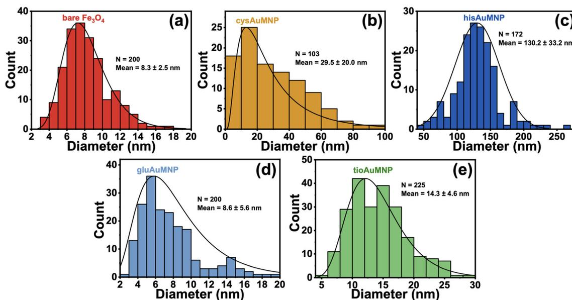
Fig. 6 Histograms obtained from STEM micrographs of the various synthesized nanoparticles. The histograms a–e correspond to: (a) bare  $\text{Fe}_3\text{O}_4$ , (b) cysAuMNP, (c) hisAuMNP, (d) gluAuMNP, and (e) tioAuMNP. All size distributions were completed using ImageJ with a minimum of 100 particles and a maximum of 225 particles per histogram.
