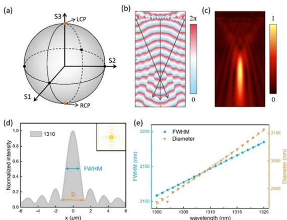
**Fig. 2** (a) Stokes parameters of the incident and outgoing light (orange dots) plotted on the Poincaré sphere. (b) and (c) Simulated phase and intensity distribution of the metasurface in the  $x$ - $z$  plane at the wavelength of 1310 nm. (d) Simulated normalized intensity line profile of the focal plane. Inset shows the focus intensity distribution. (e) Plot of simulated FWHM (blue) and diameter (orange) as a function of wavelength from 1300 to 1320 nm.
