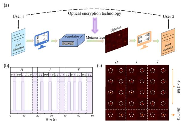
**Fig. 4** (a) Schematic diagram of the optical encryption system based on the designed metasurface optical element. (b) The input and output signals of converting ASCII code “HIT” in the optical encryption system. There is a delimiter code “11” between the letters. (c) Simulated optical ciphertext of secret information “HIT”.
